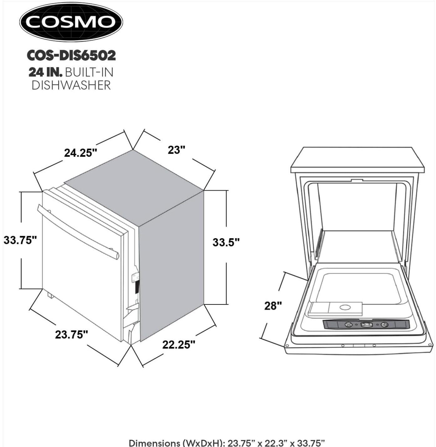
Figure 3.3.1: COSMO COS-DIS6502 Dishwasher Dimensions. Width: 23.75 inches, Depth: 22.25 inches, Height: 33.75 inches.
