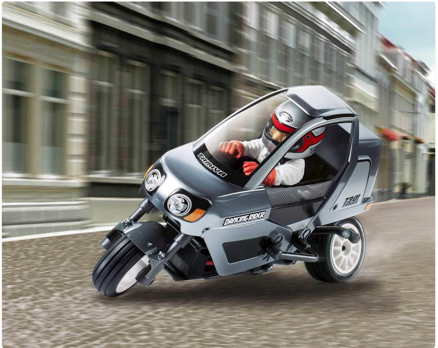
Figure 2.2: The Dancing Rider Trike demonstrating its leaning capability during a turn.
