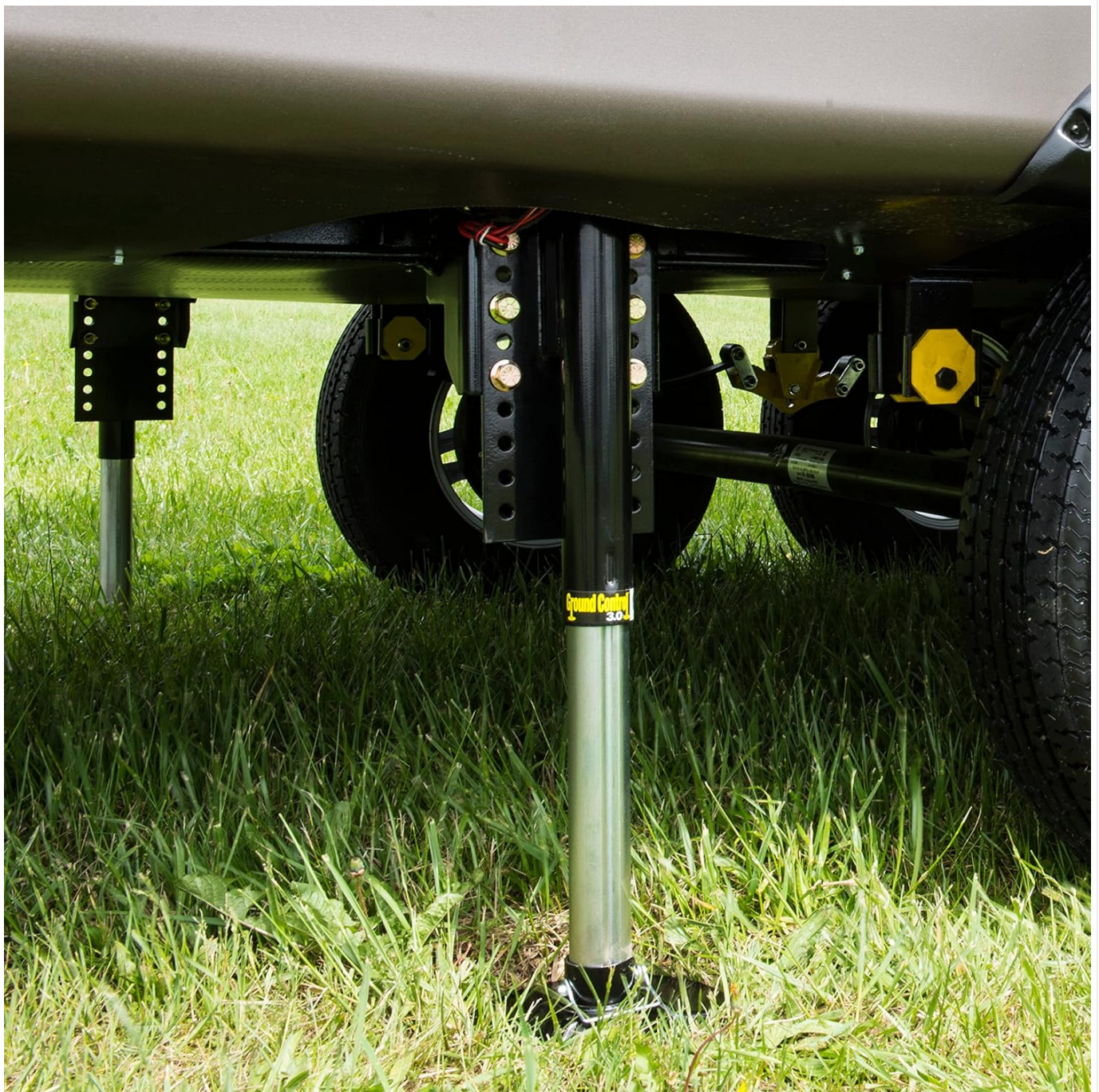
Figure 5: Jack in Operation. This image shows the jack extended, providing stabilization to a 5th wheel RV, demonstrating its function in a real-world setting.
