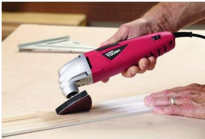
Image: A user demonstrating the use of the Hyper Tough AQ60003G multi-tool for sanding a wooden surface, highlighting the ergonomic grip and compact design.
