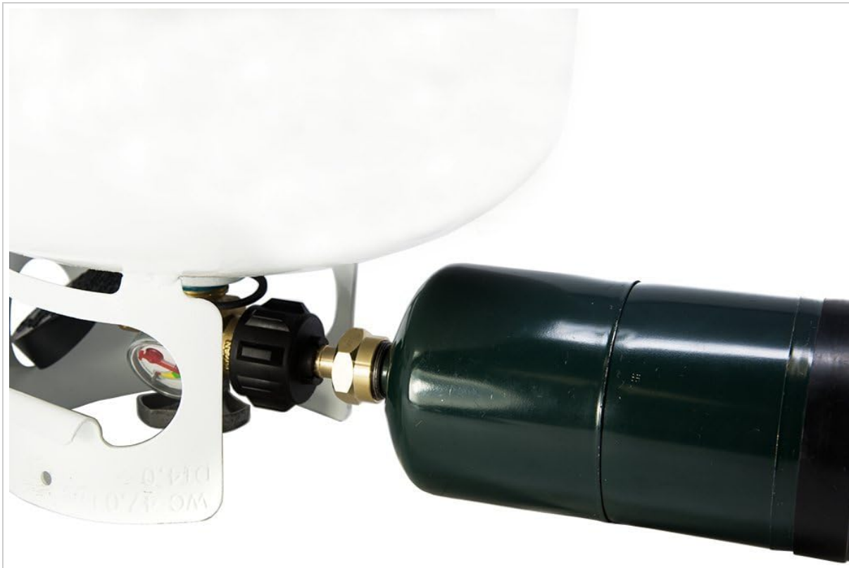
Image: Close-up of the adapter during the refilling process, with the 20lb tank inverted above the 1lb tank.
