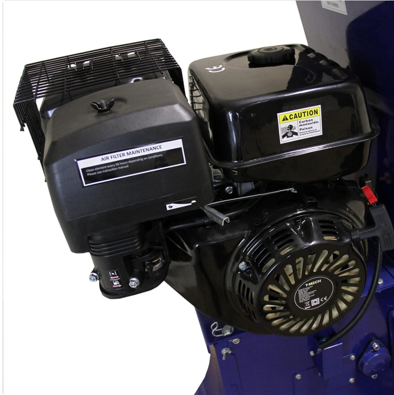
Figure 2.2: Engine detail, showing the air filter housing and fuel cap.
