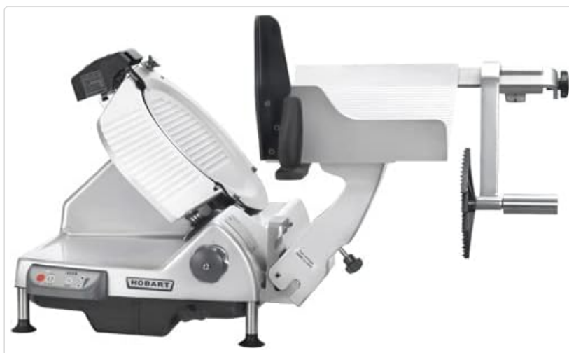
Figure 5: The removable carriage system allows for thorough cleaning.
