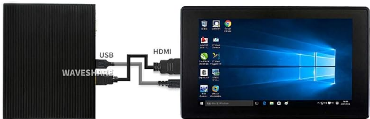
Figure 4.2: Visual guide for connecting the 7-inch monitor to a Raspberry Pi, showing HDMI and USB connections.
