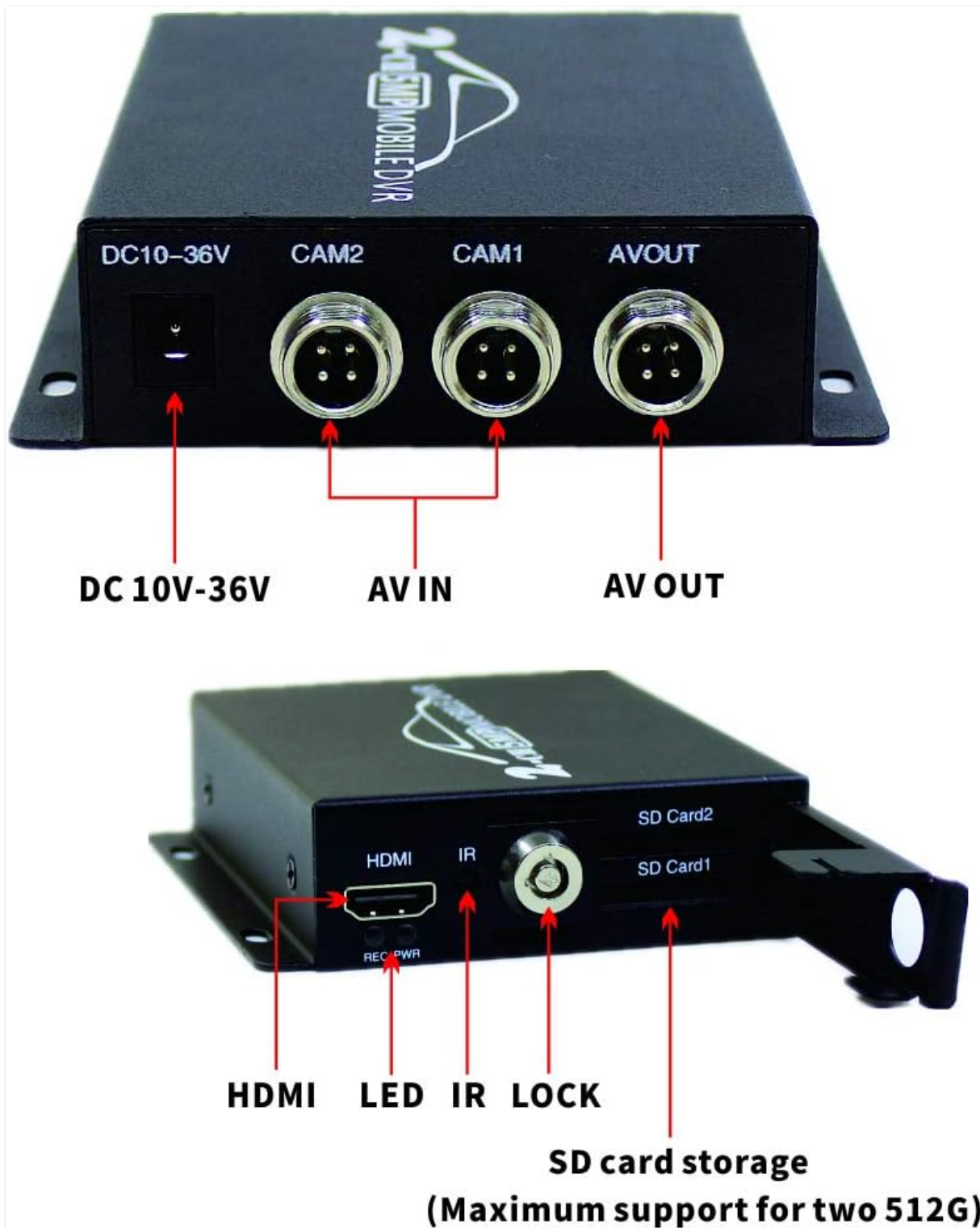
Image: A detailed view of the Mobile DVR unit, highlighting the DC power input, CAM1 and CAM2 video inputs, AV OUT port, HDMI output, IR receiver, REC/PWR indicators, and dual SD card slots.
