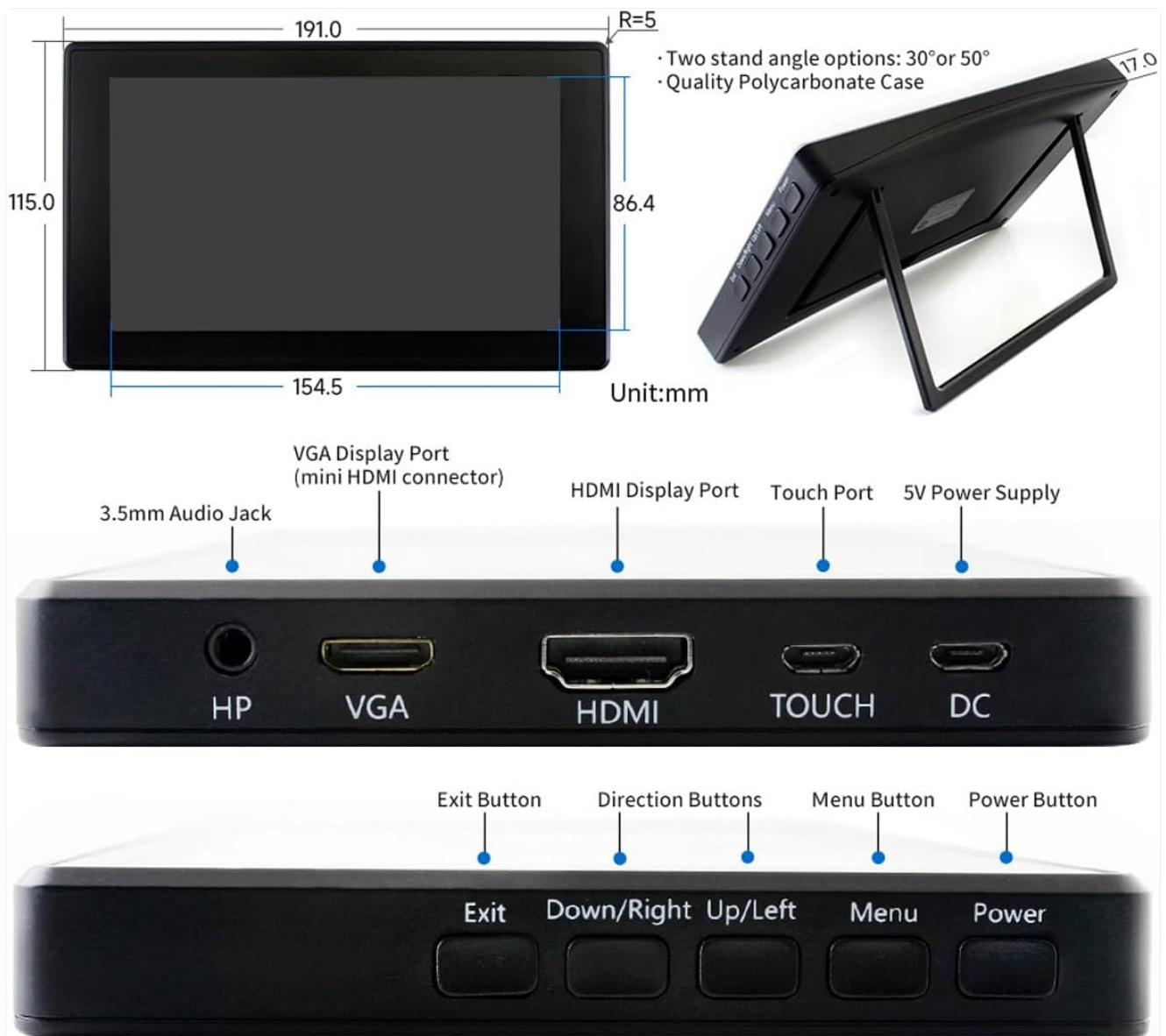
Image: Detailed view of the Waveshare 7-inch LCD's appearance, including its dimensions, and labeled ports (3.5mm Audio Jack, VGA Display Port, HDMI Display Port, Touch Port, 5V Power Supply) and control buttons (Exit, Down/Right, Up/Left, Menu, Power).
