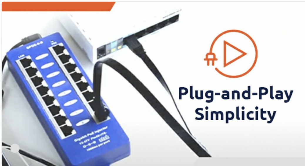
Figure 4: Illustration of the GPOE-8B's plug-and-play setup, showing connections between a network switch, the injector, and a powered device.
