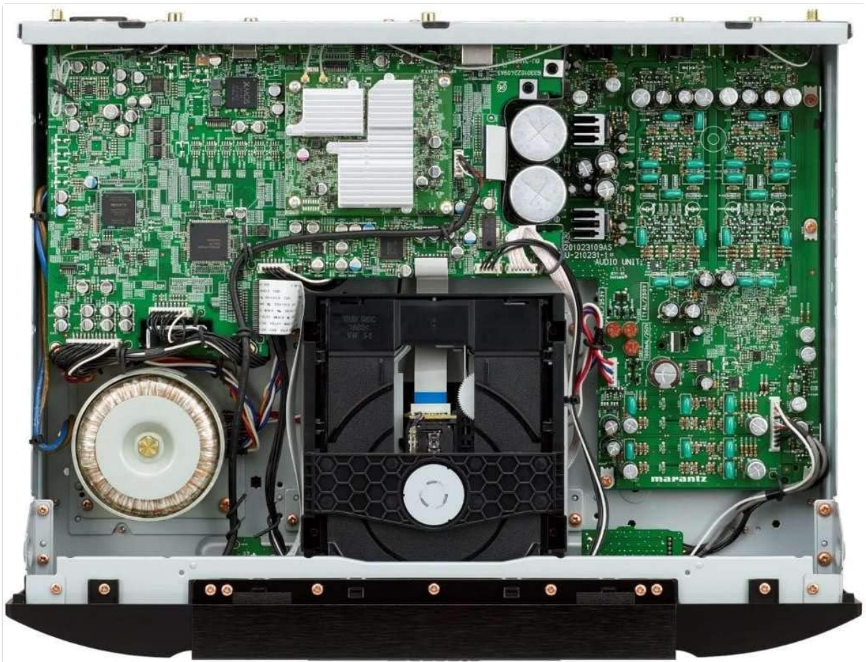
Figure 4: Internal view showcasing the components of the Marantz ND8006.
