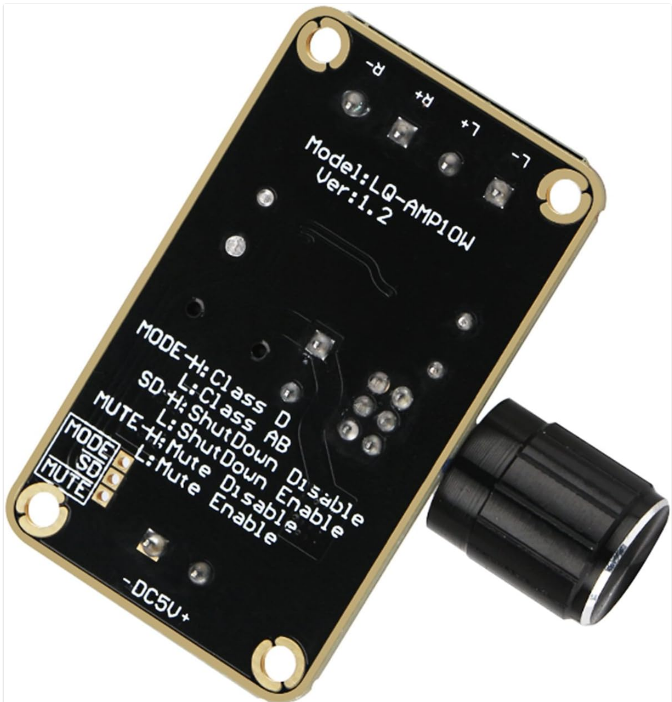
Figure 4.2: Amplifier Board Bottom View with Mode Settings
