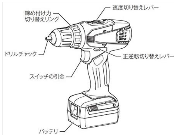
Figure 3.1: Main Components of the Driver Drill
