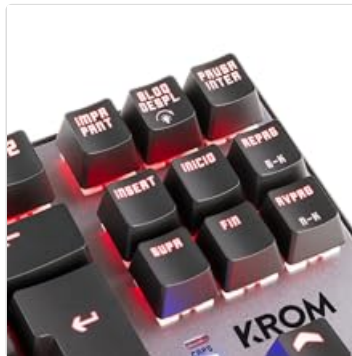
Image 3.2: A close-up view of the KROM Kernel TKL keyboard's keycaps, clearly showing the Spanish QWERTY layout and secondary functions.
