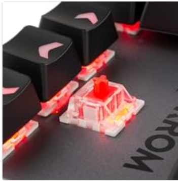
Image 4.2: A close-up image showing a mechanical switch on the KROM Kernel TKL keyboard, highlighting its design and potential for easy replacement (CIY Technology).
