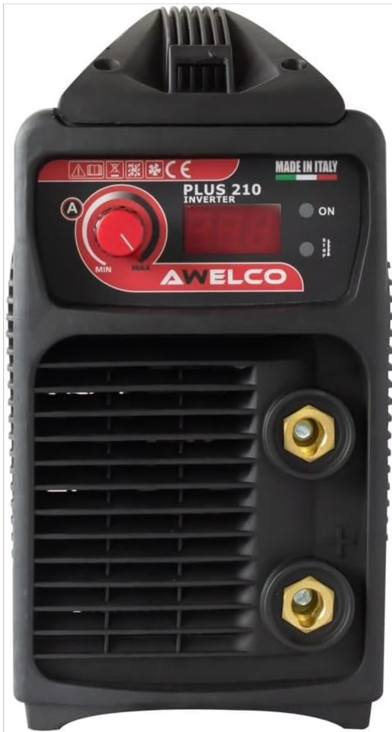
Figure 3: Front view showing the quick-connect terminals for welding cables. The top terminal is typically for the electrode holder, and the bottom for the ground clamp, depending on polarity requirements.
