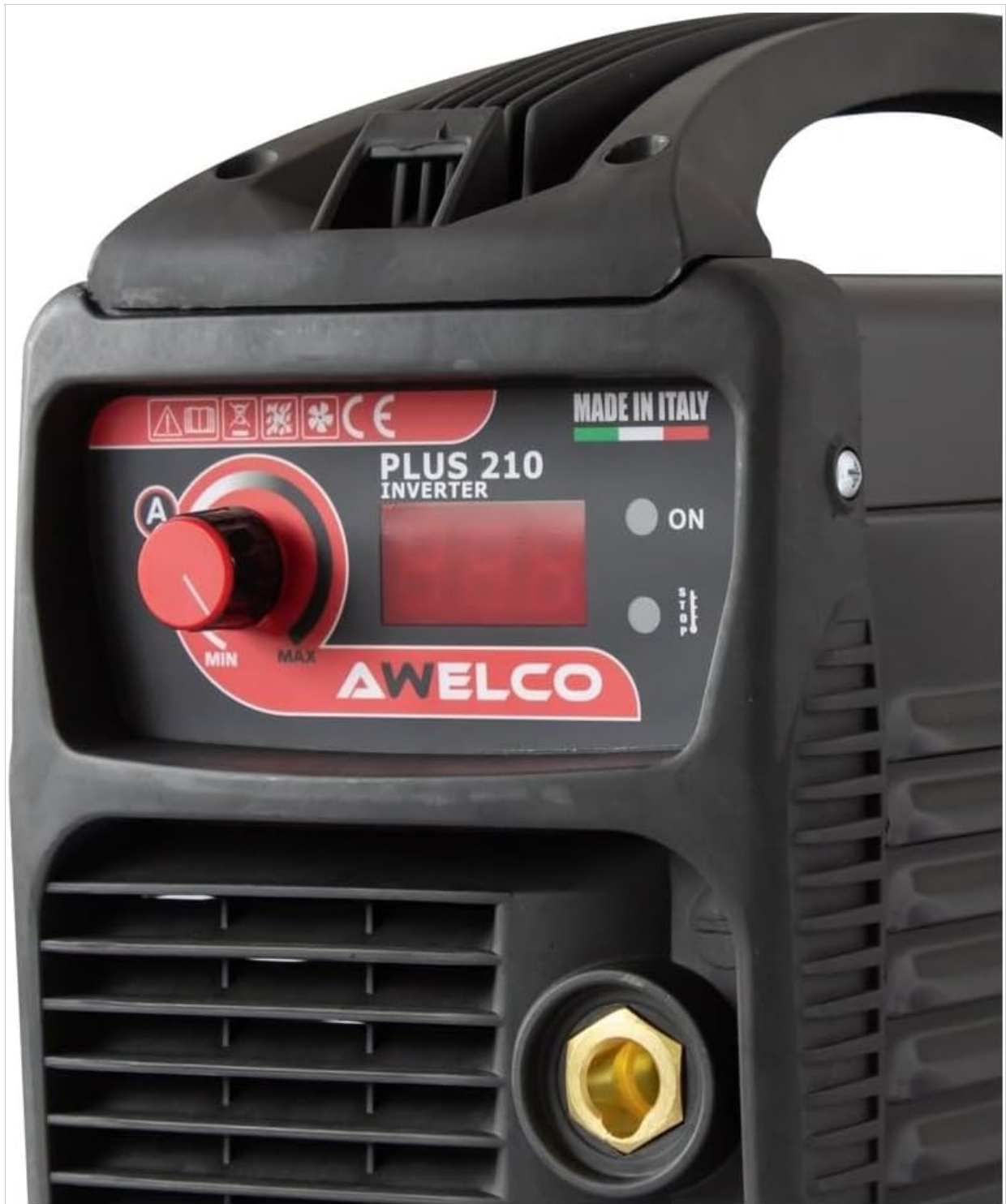
Figure 2: Close-up of the control panel. Features include the amperage adjustment knob (MIN-MAX), digital display, power indicator light (ON), and thermal overload indicator.
