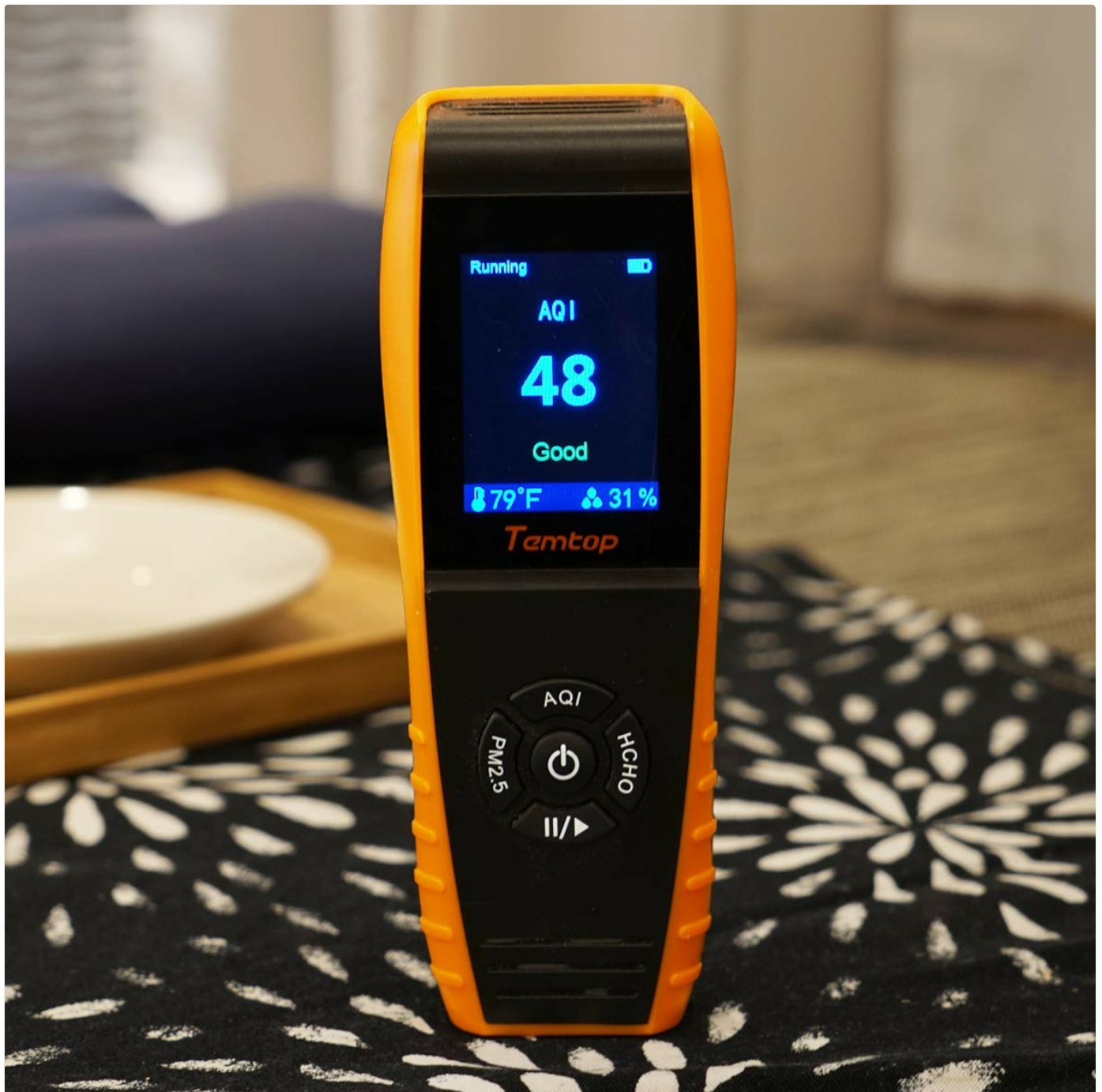
Figure 5: The device display showing AQI (48, Good), temperature (79°F), and humidity (31%).
