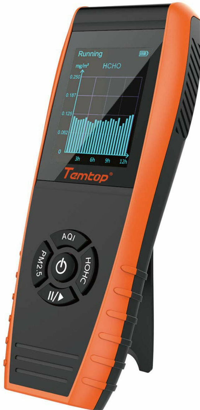
Figure 6: The device displaying a histogram of HCHO levels over time, with its integrated kickstand extended for viewing.
