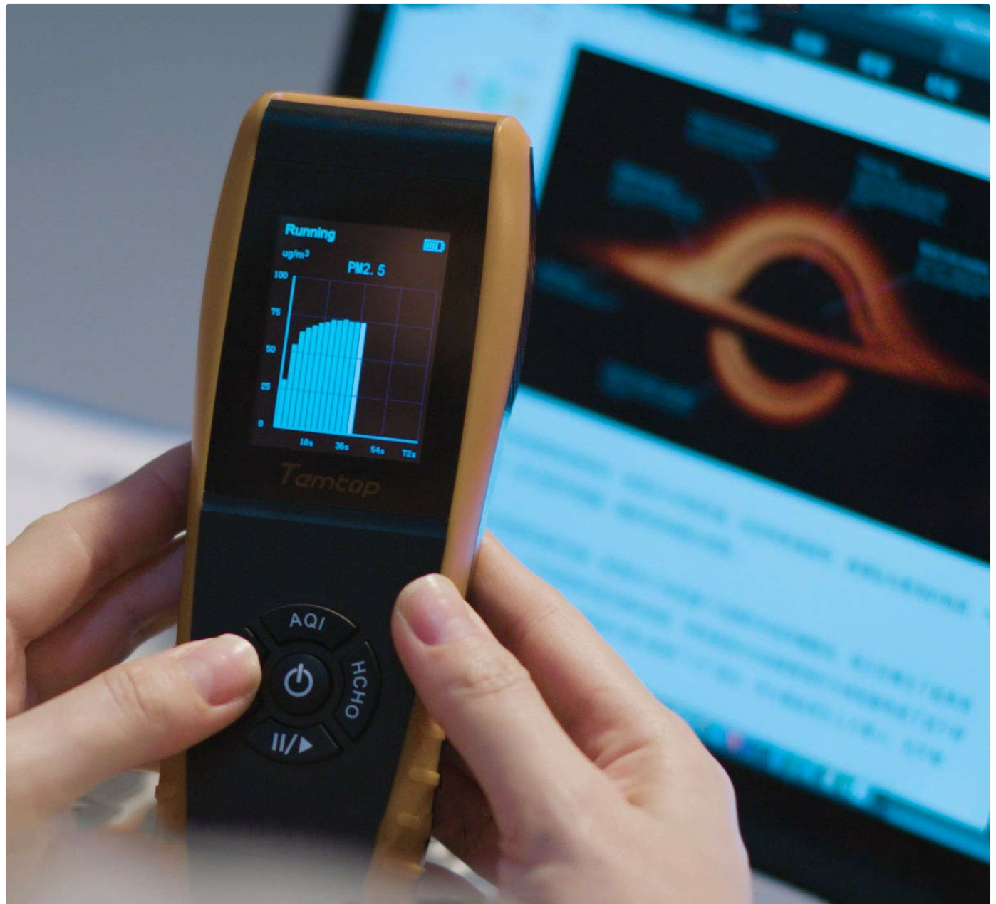
Figure 8: The device in use, showing a PM2.5 histogram on its screen, indicating air quality trends.
