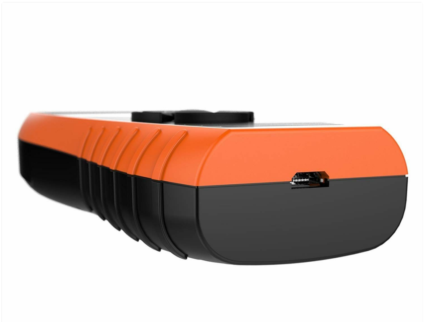
Figure 4: Bottom view of the Temtop LKC-1000S+ showing the micro-USB charging port. Note that the device cannot stand upright on its kickstand while charging due to the port's location.
