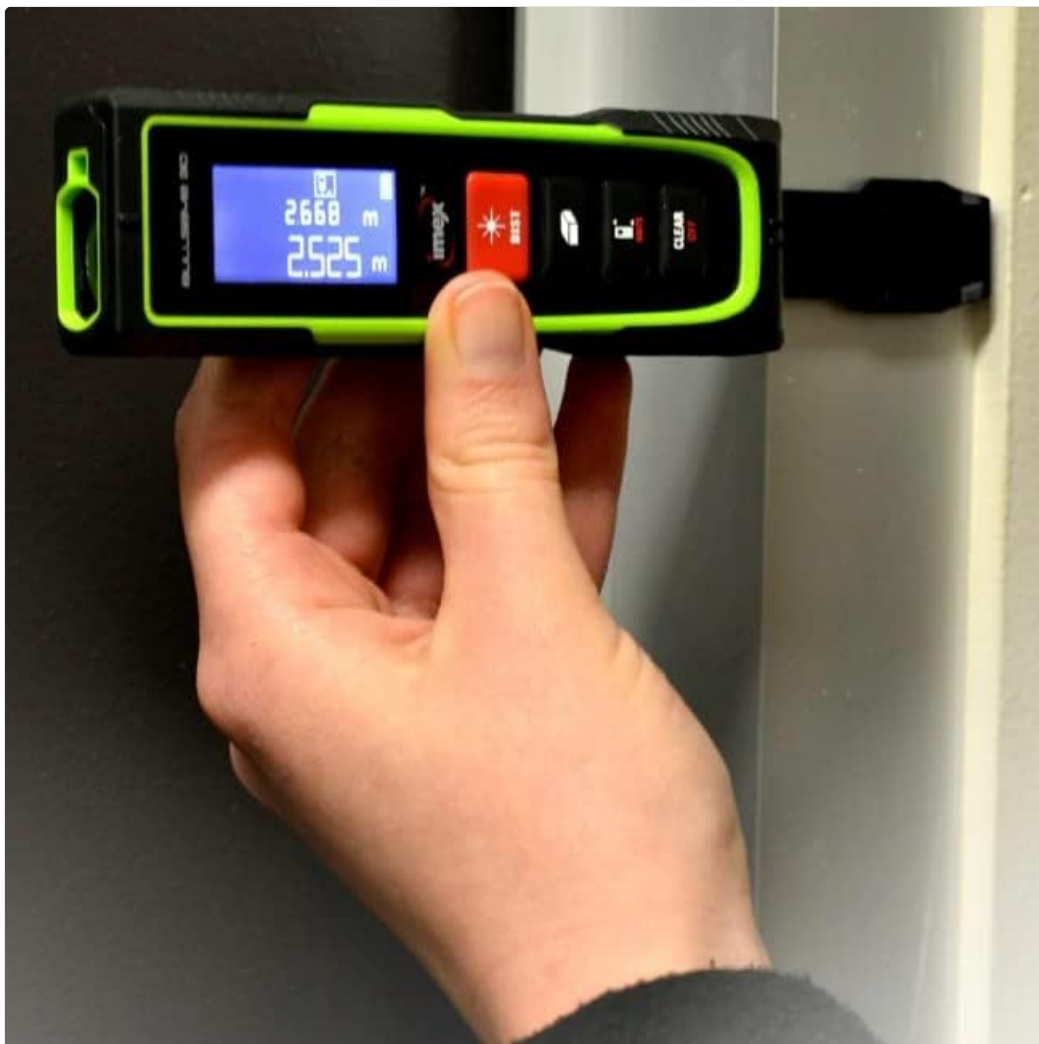
Figure 6.1: The Imex Bullseye 30 being used to measure a distance, showing the display with measurement readings.
