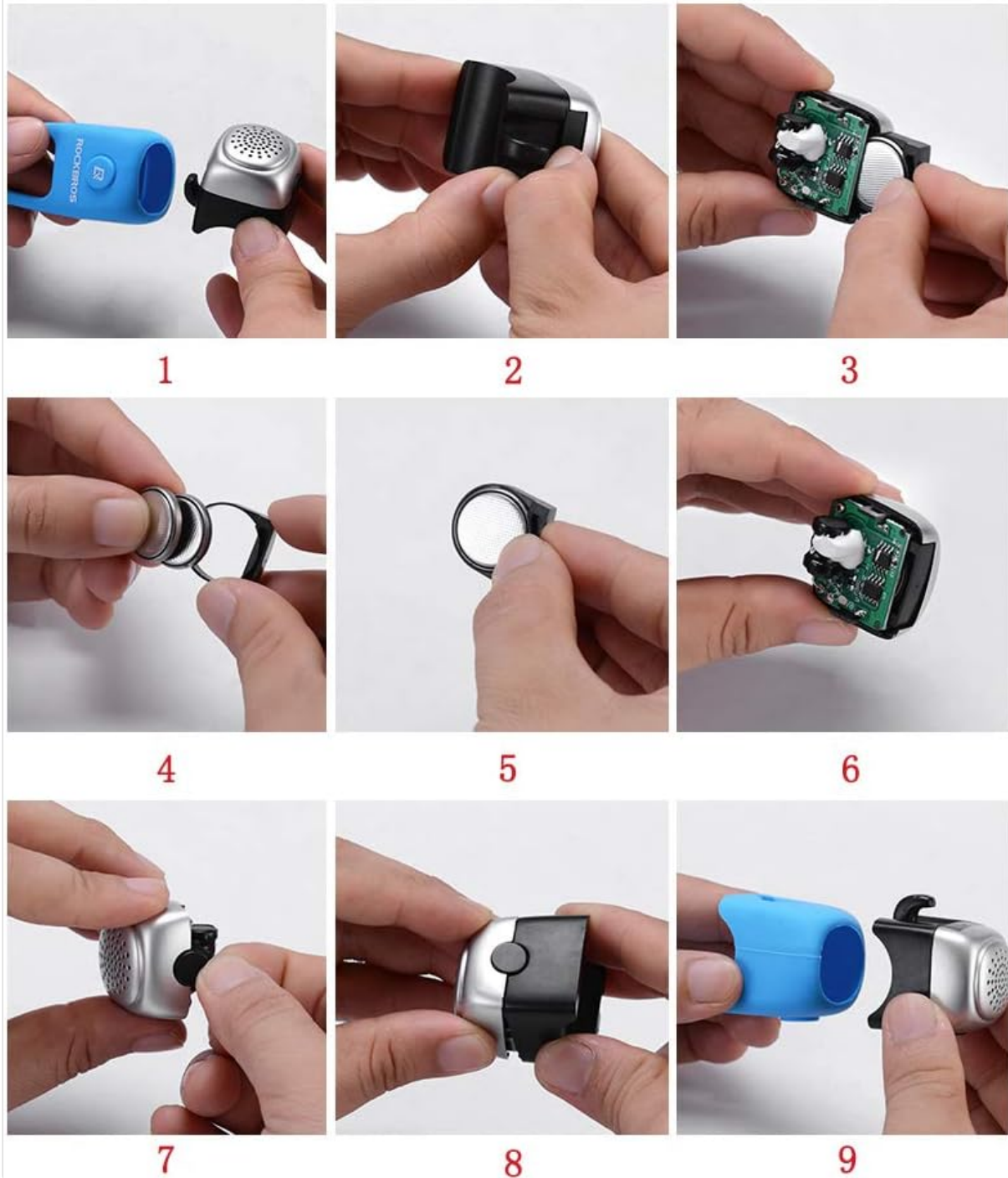
Figure 5.1: Battery replacement steps.
