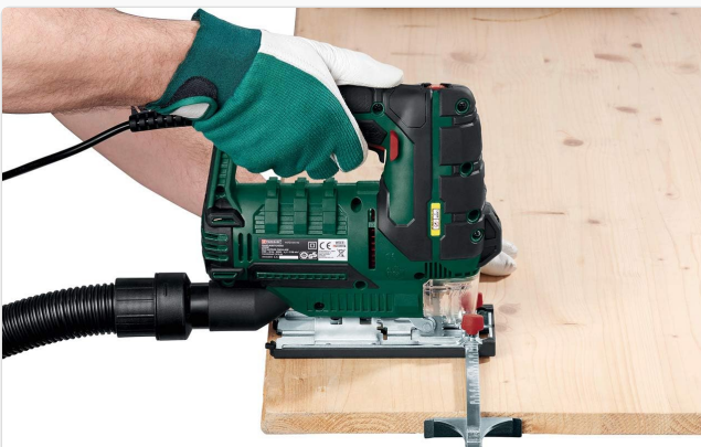
Figure 4.4: The jigsaw connected to an external dust extraction hose, demonstrating how to maintain a clean cutting line and work area.
