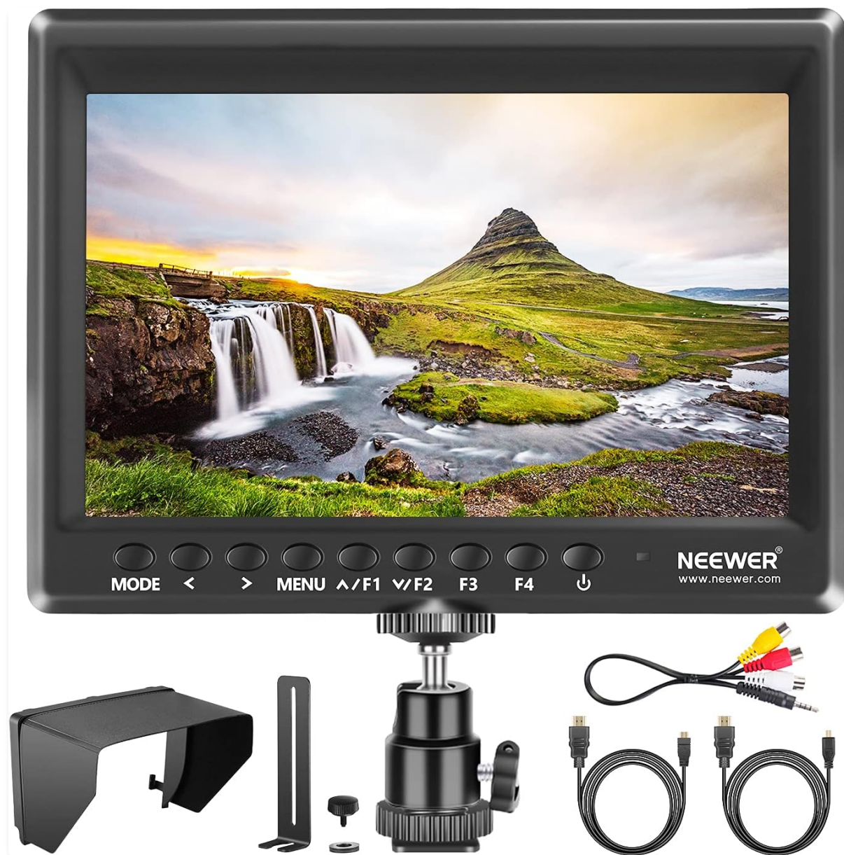
Image 1.1: NEEWER F100 7-inch Camera Field Monitor and its accessories, including sunshade, ball head, and various HDMI cables.
