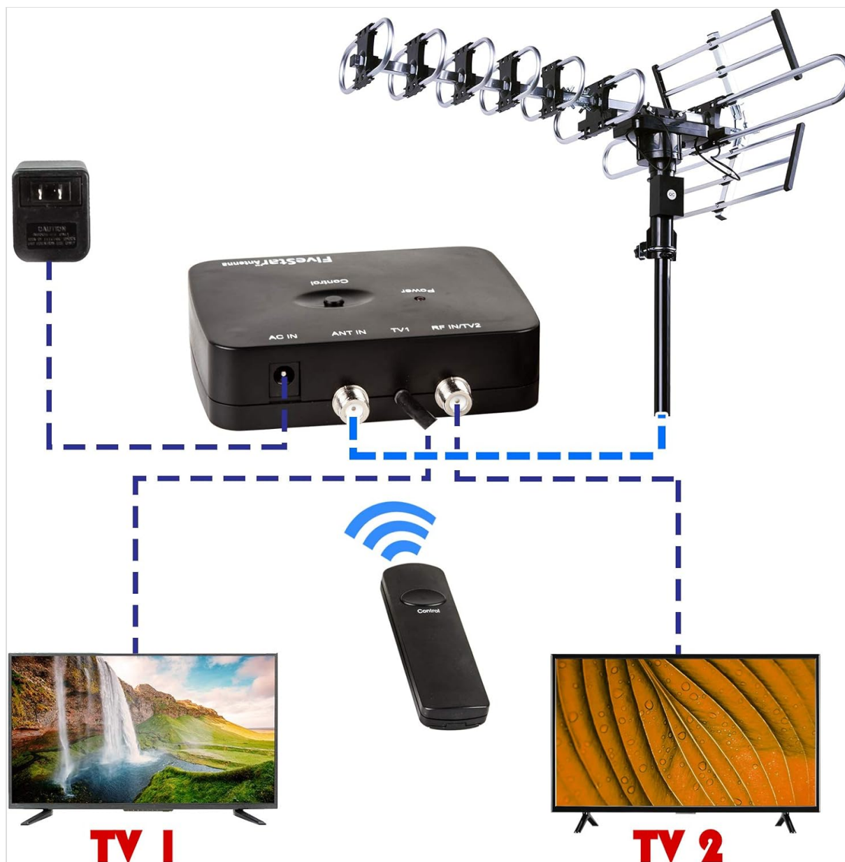
Image 5.1: Diagram illustrating how to connect the antenna to the control box and then to one or two televisions.
