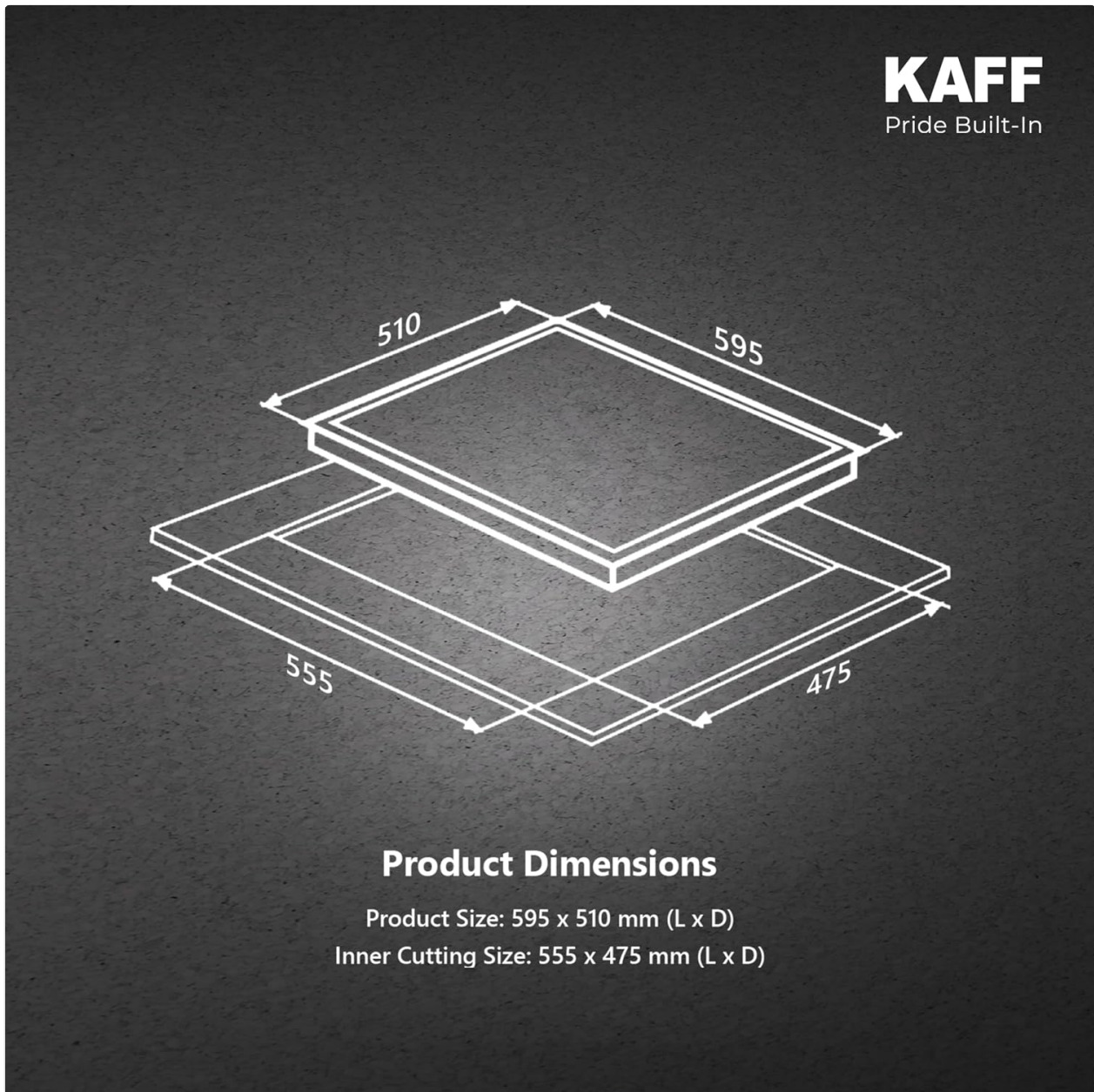
Figure 3: Installation diagram showing the required countertop cut-out dimensions and clearances for the KAFF NE4B60SS hob.
