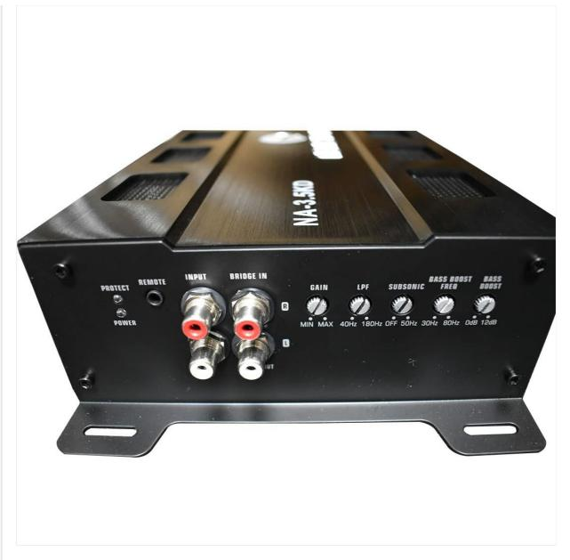
**Figure 3:** View of the input and control panel side of the NA-3.5KD amplifier. Features include PROTECT and POWER indicator LEDs, REMOTE port, RCA INPUTs, BRIDGE IN, GAIN control, LPF (Low Pass Filter) control, SUBSONIC filter control, BASS BOOST FREQ, and BASS BOOST level controls.
