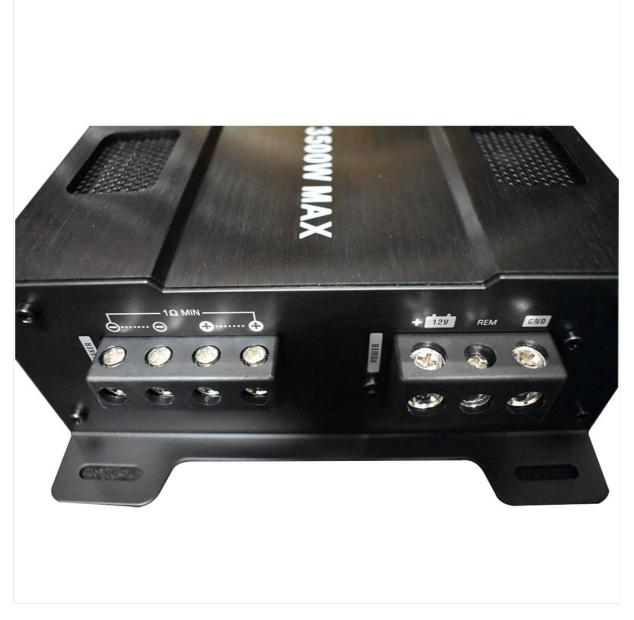
Figure 2: View of the power and speaker terminal side of the NA-3.5KD amplifier. This side includes terminals for BATT+ (12V), REM (Remote Turn-On), GND (Ground), and speaker outputs with a  $1\Omega$  minimum impedance rating.
