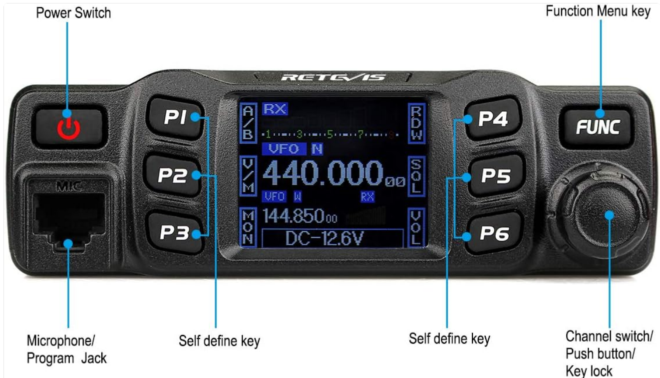
Figure 3: Front Panel Controls. This diagram labels the Power Switch, P1-P6 programmable keys, Microphone/Program Jack, Self-define keys, Function Menu key, and Channel switch/ Push button/ Key lock.
