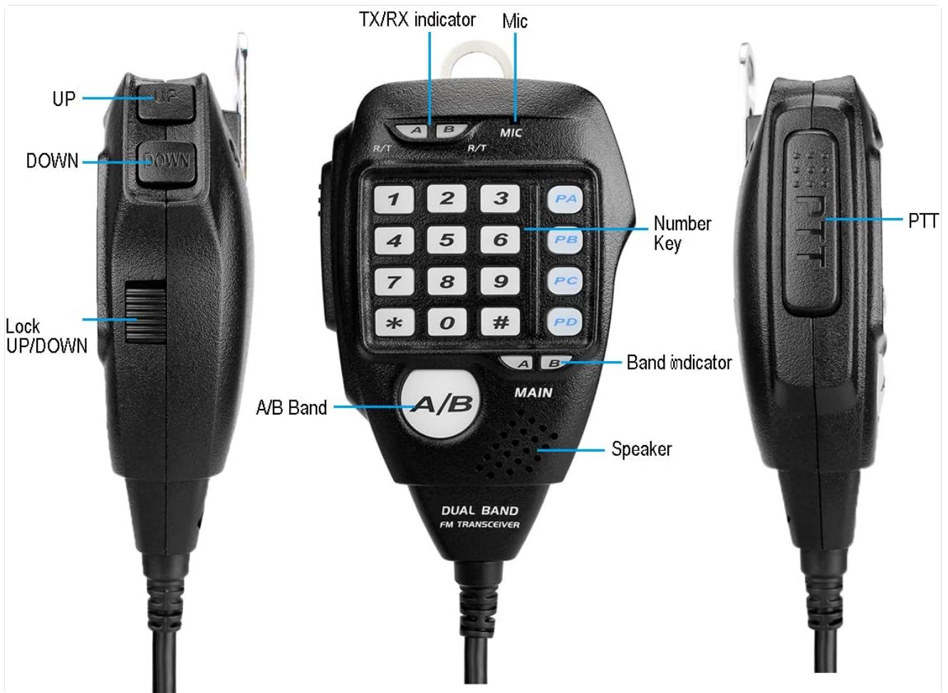
Figure 4: Handheld Microphone Controls. This diagram labels the UP/DOWN buttons, Lock UP/DOWN switch, TX/RX indicator, Mic, Number Keypad, Band indicator, Speaker, A/B Band button, and PTT (Push-To-Talk) button.
