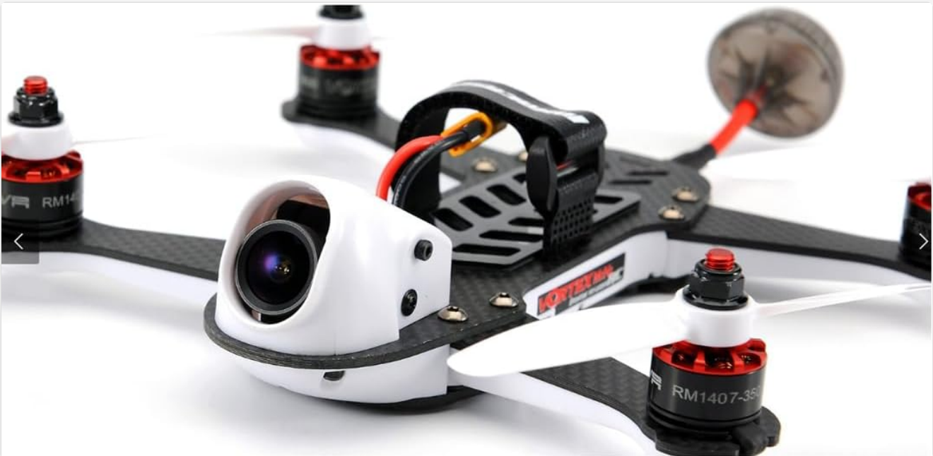
Figure 4: Front camera of the Vortex 180, essential for FPV flight.
