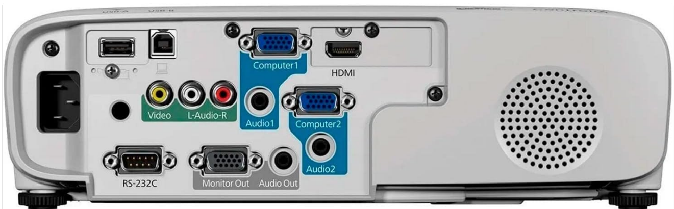
Image: Rear panel of the Epson PowerLite S39 projector, displaying available connectivity ports.
