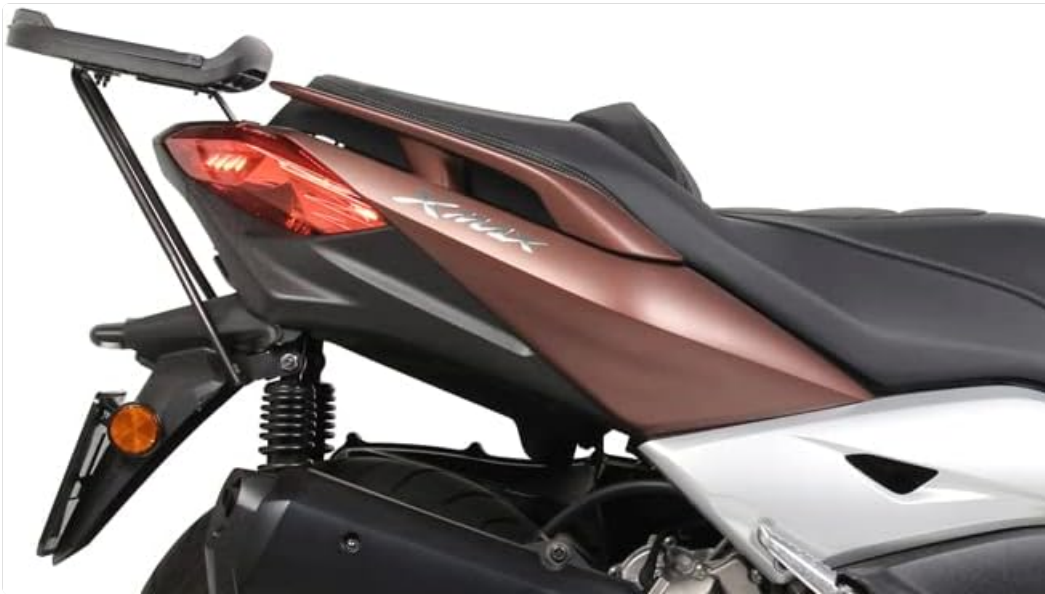
Image 4.1: Detailed view of the SHAD Top Master Kit brackets installed on a Yamaha X-MAX scooter.
