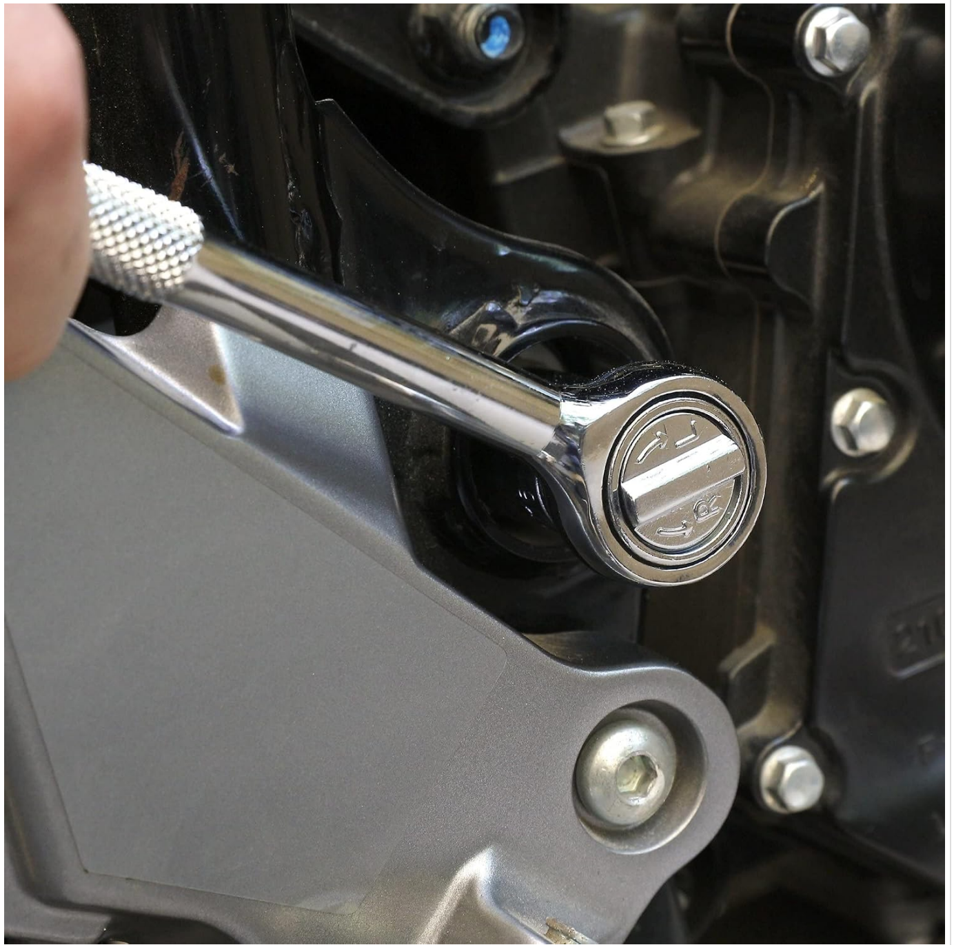
Figure 5: Applying the ratchet and socket to a component for tightening or loosening.
