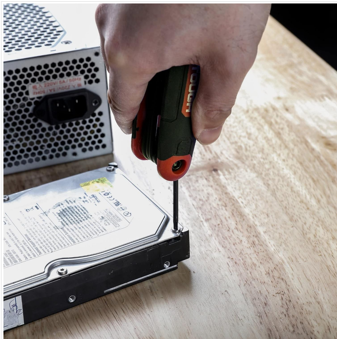
Figure 9: Using a star key to work on a component with a star-shaped screw head.
