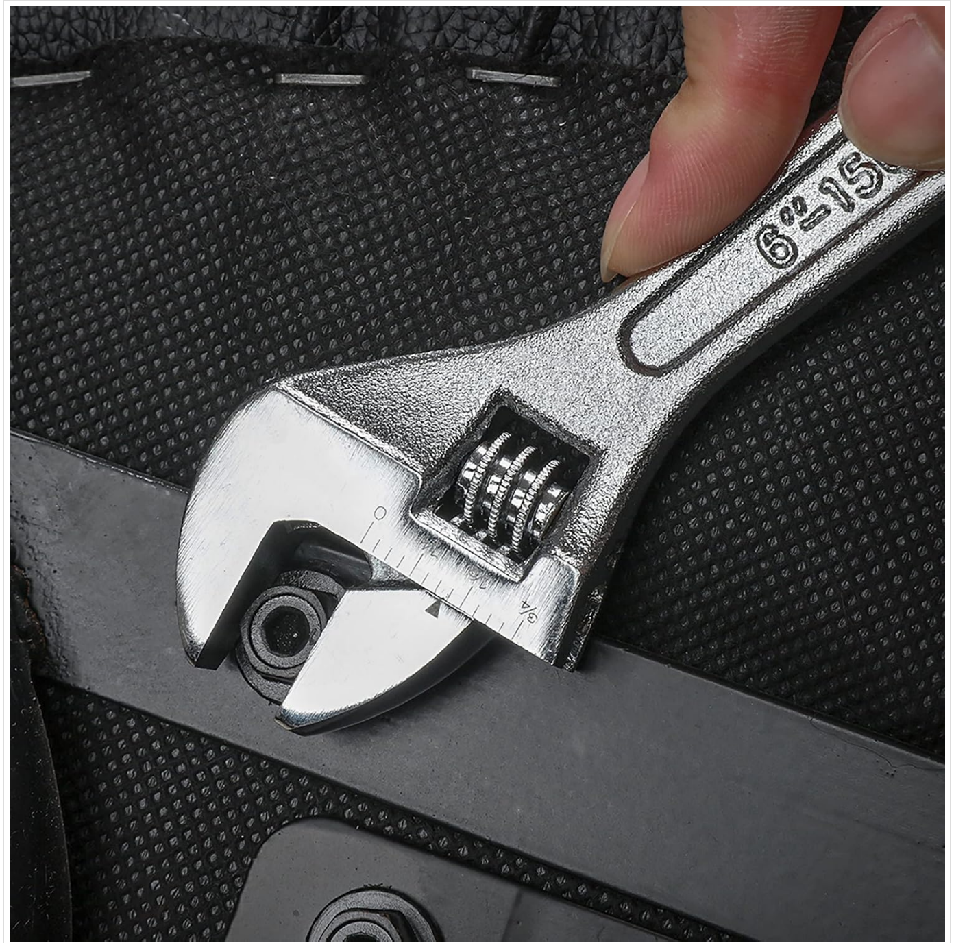
Figure 3: Proper use of the adjustable wrench for securing or loosening fasteners.
