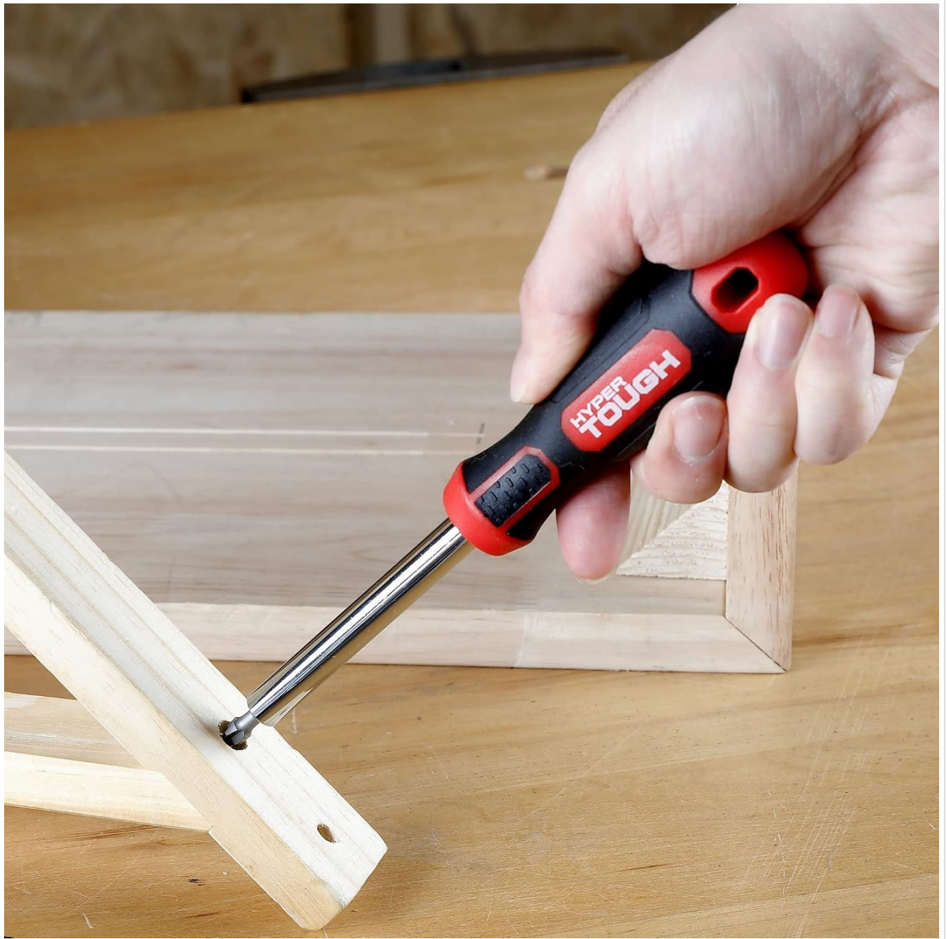
Figure 7: The magnetic screwdriver handle in use for driving a screw.
