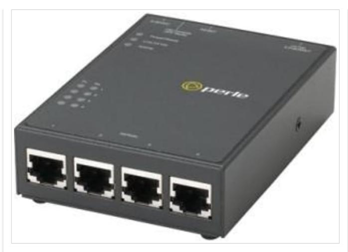
This image displays the Perle IOLAN STS4D GR Secure Terminal Server. The device is a compact, dark gray rectangular unit. The front panel features four RJ-45 serial ports, clearly visible at the bottom. The top surface shows LED indicators for power, network activity, and serial port status, along with the 'Perle' logo.
