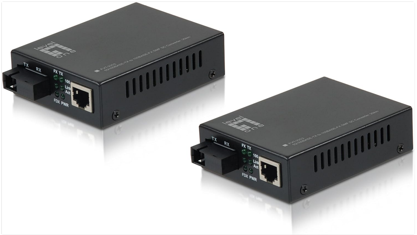
Figure 3.1: Front view of the LevelOne FVT-2202 Media Converter, showing the RJ45 Ethernet port, SC fiber optic port, and LED indicators for TX, RX, Link/Act, and Power.
