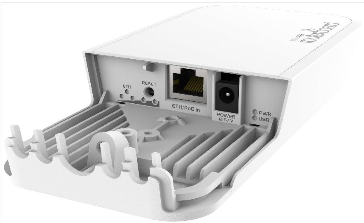
Image 3.2: Detailed view of the wAP60G device's underside, showing the Ethernet/PoE In port, power input, reset button, and mounting points.
