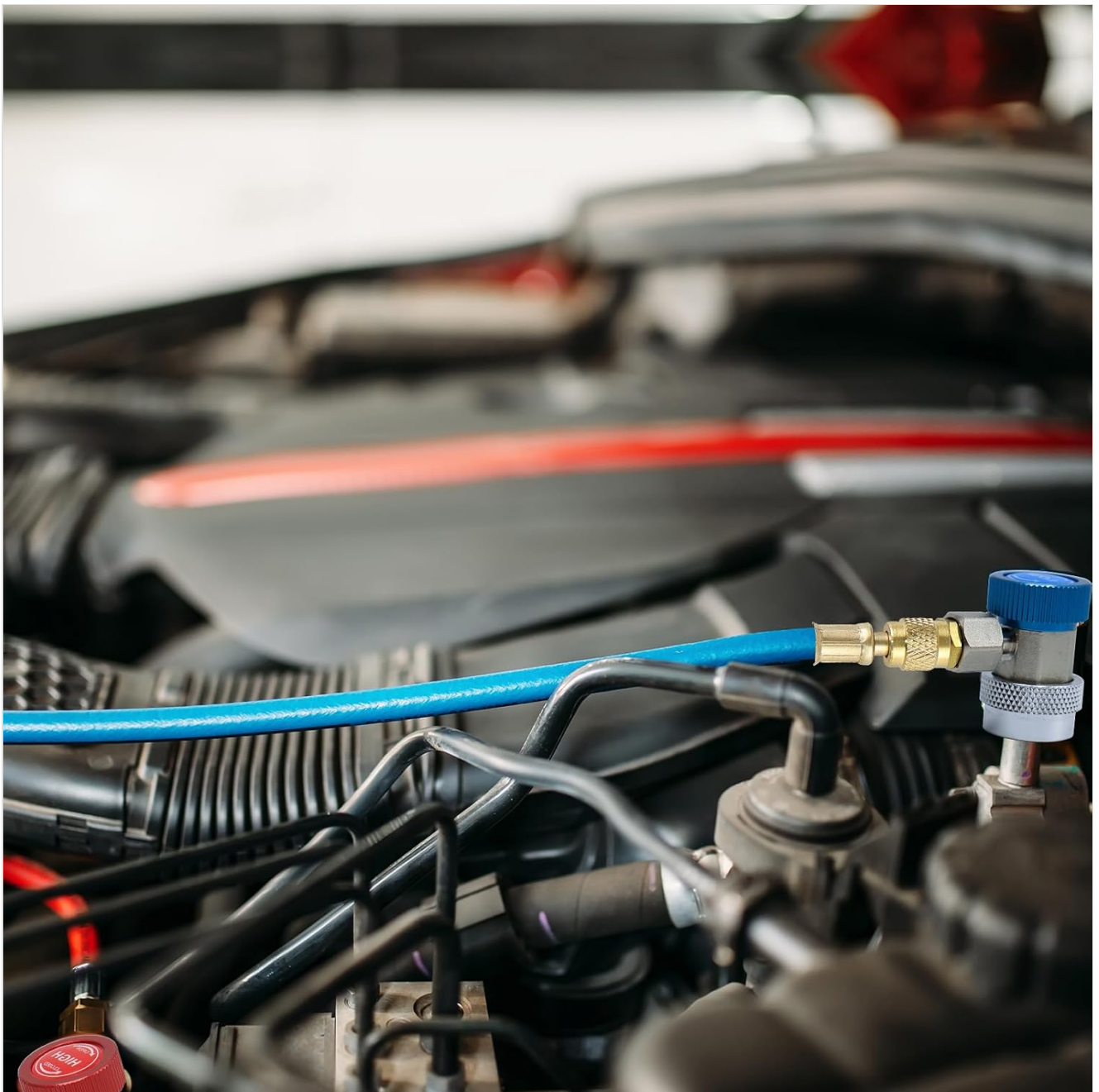
Image: A close-up view of the blue quick coupler attached to the low-pressure service port of a vehicle's air conditioning system.
