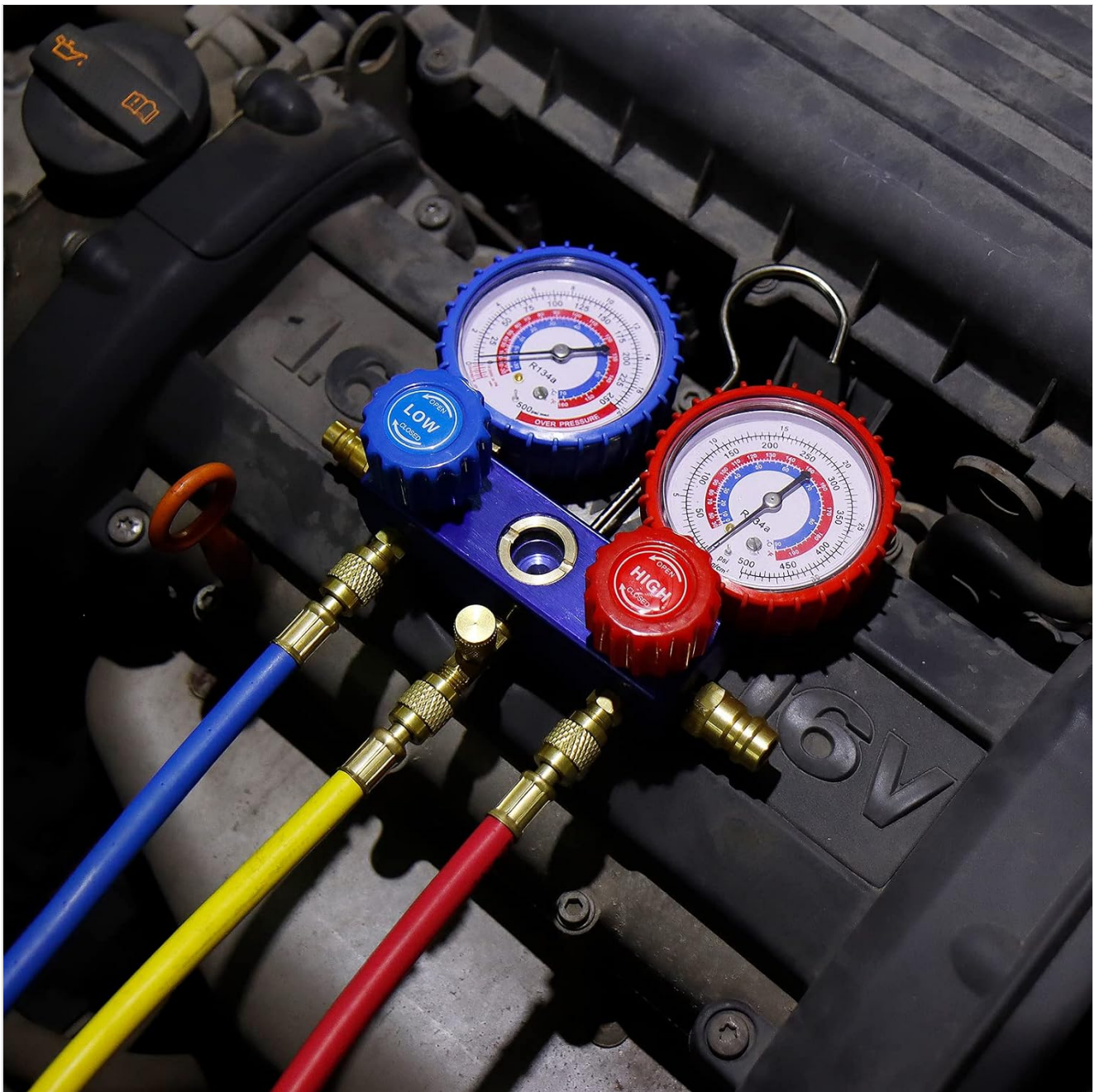
Image: The manifold gauge set with hoses and quick couplers connected to the service ports of a car's air conditioning system, located within the engine bay.
