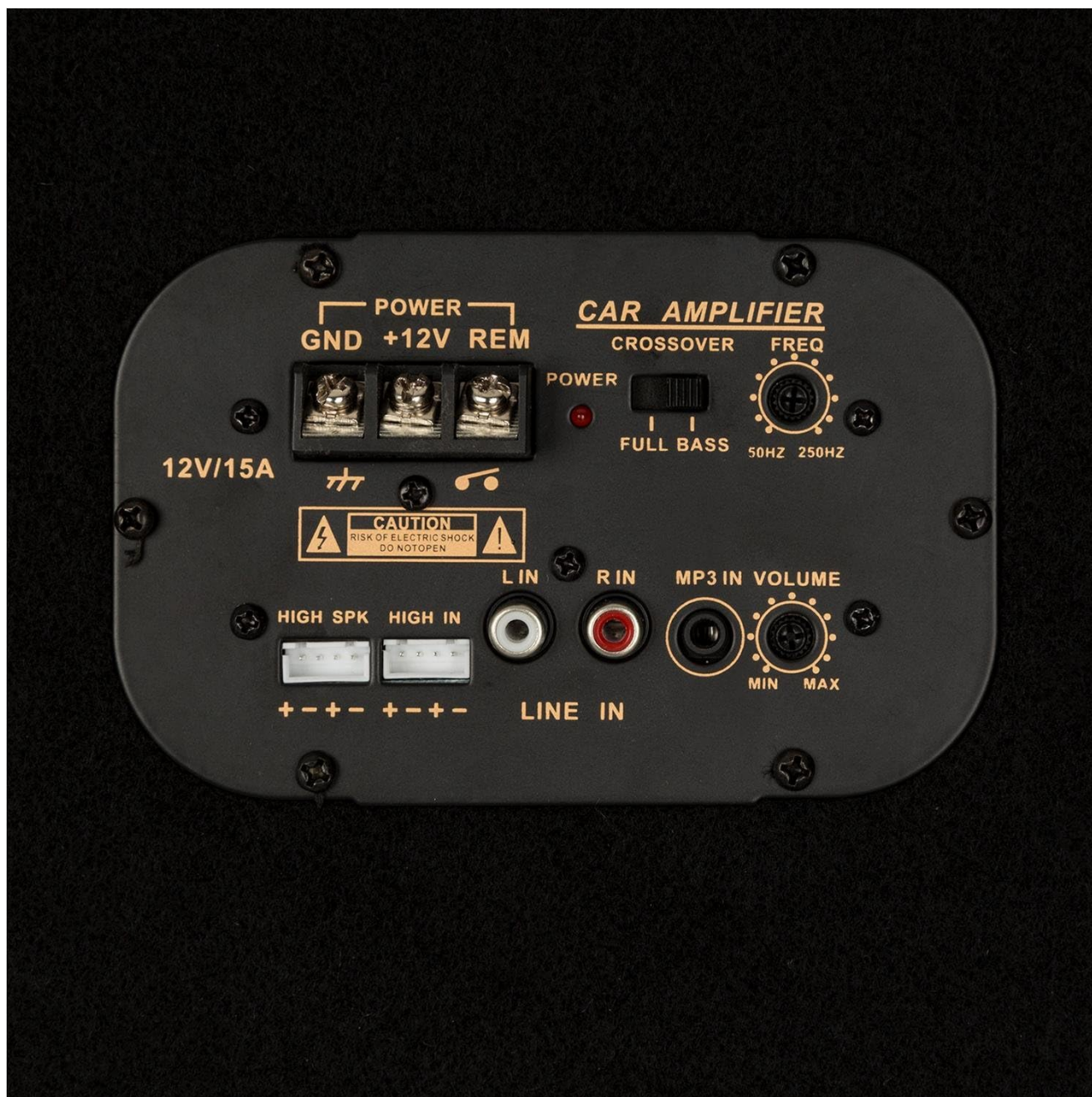
Figure 4.3: Rear panel of the subwoofer, showing power terminals, high-level input, RCA line inputs, MP3 input, volume control, crossover switch, and frequency adjustment knob.
