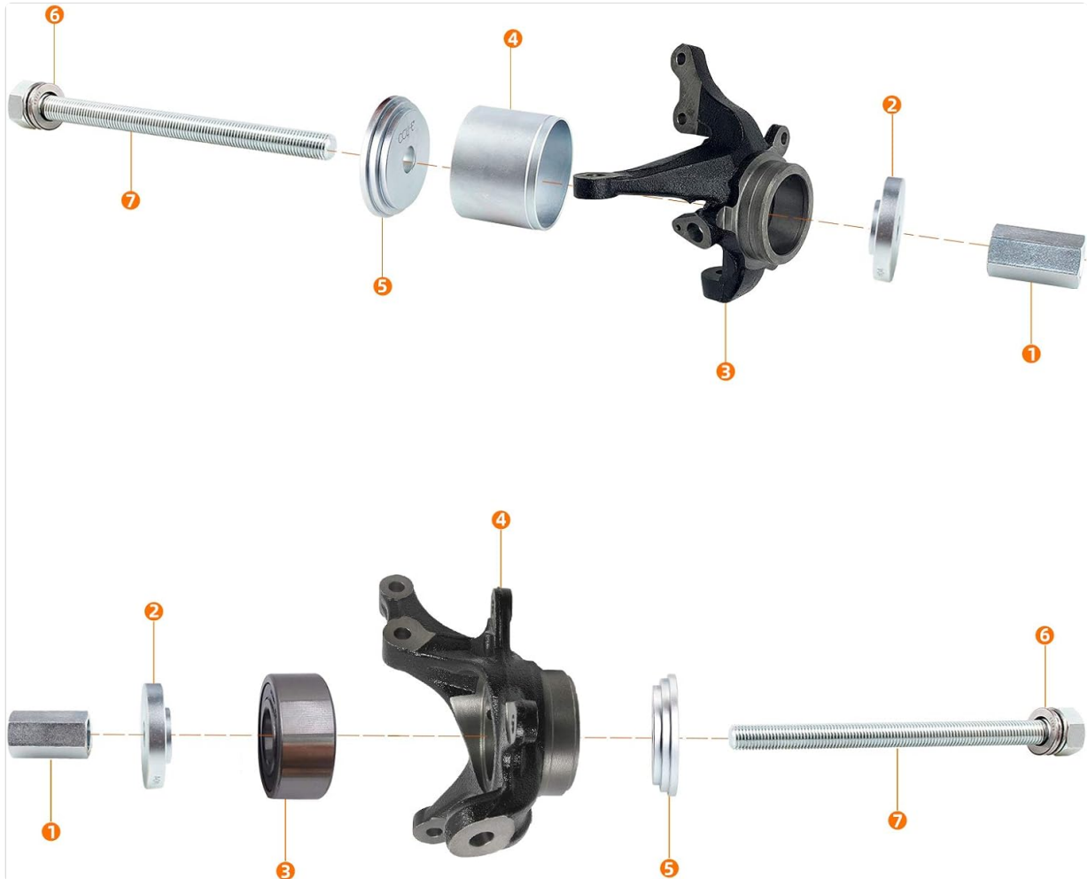
Image 3: Exploded view illustrating the setup for wheel bearing removal.
