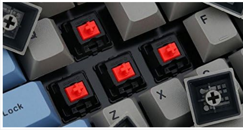
Figure 5: View of Cherry MX switches, illustrating the mechanical components.
