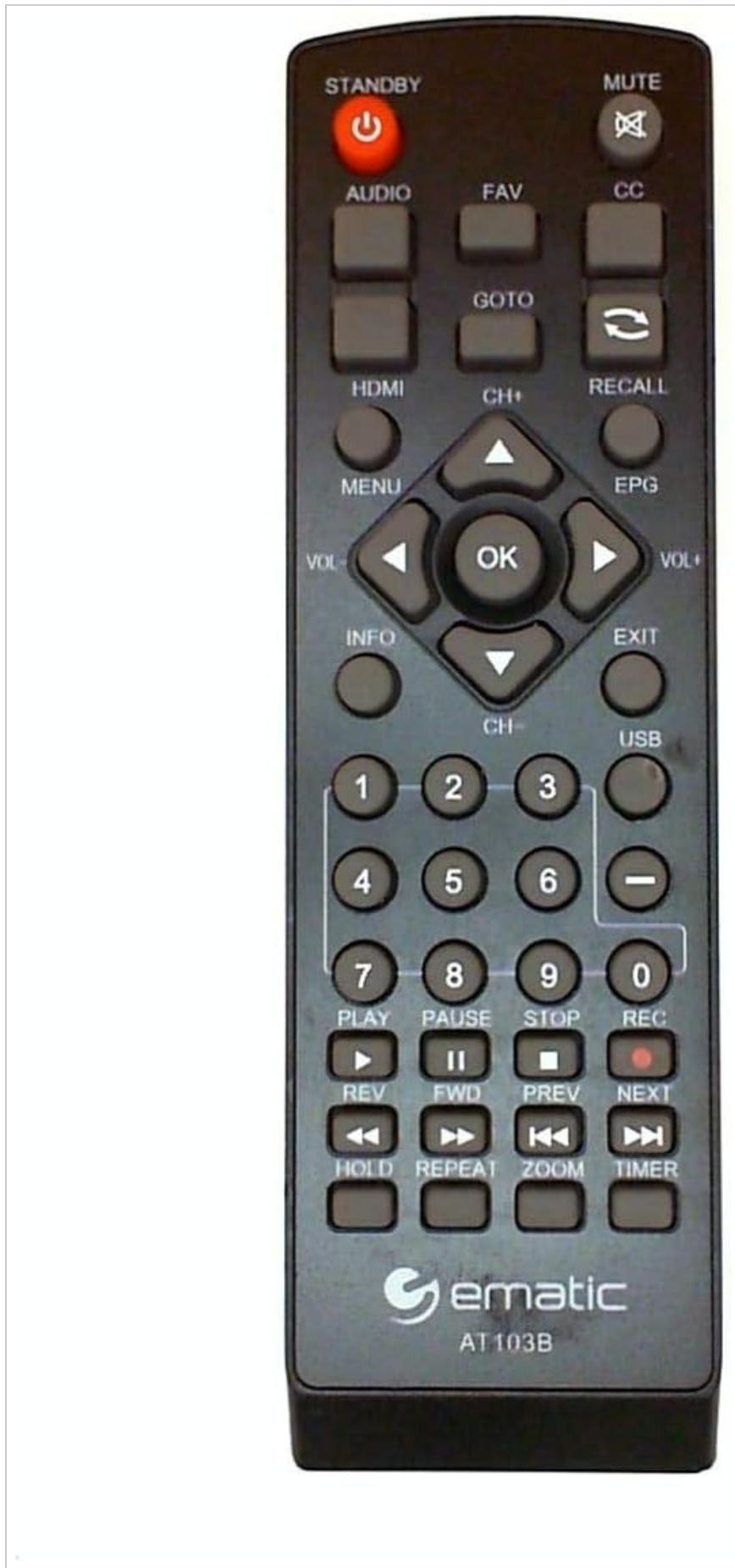
**Figure 2.1:** Ematic AT103B Remote Control. This image displays the full remote control, featuring a black body with gray buttons. Key buttons include Power (red), Mute, Audio, Channel Up/Down, Volume Up/Down, Numeric keypad, and media playback controls.
