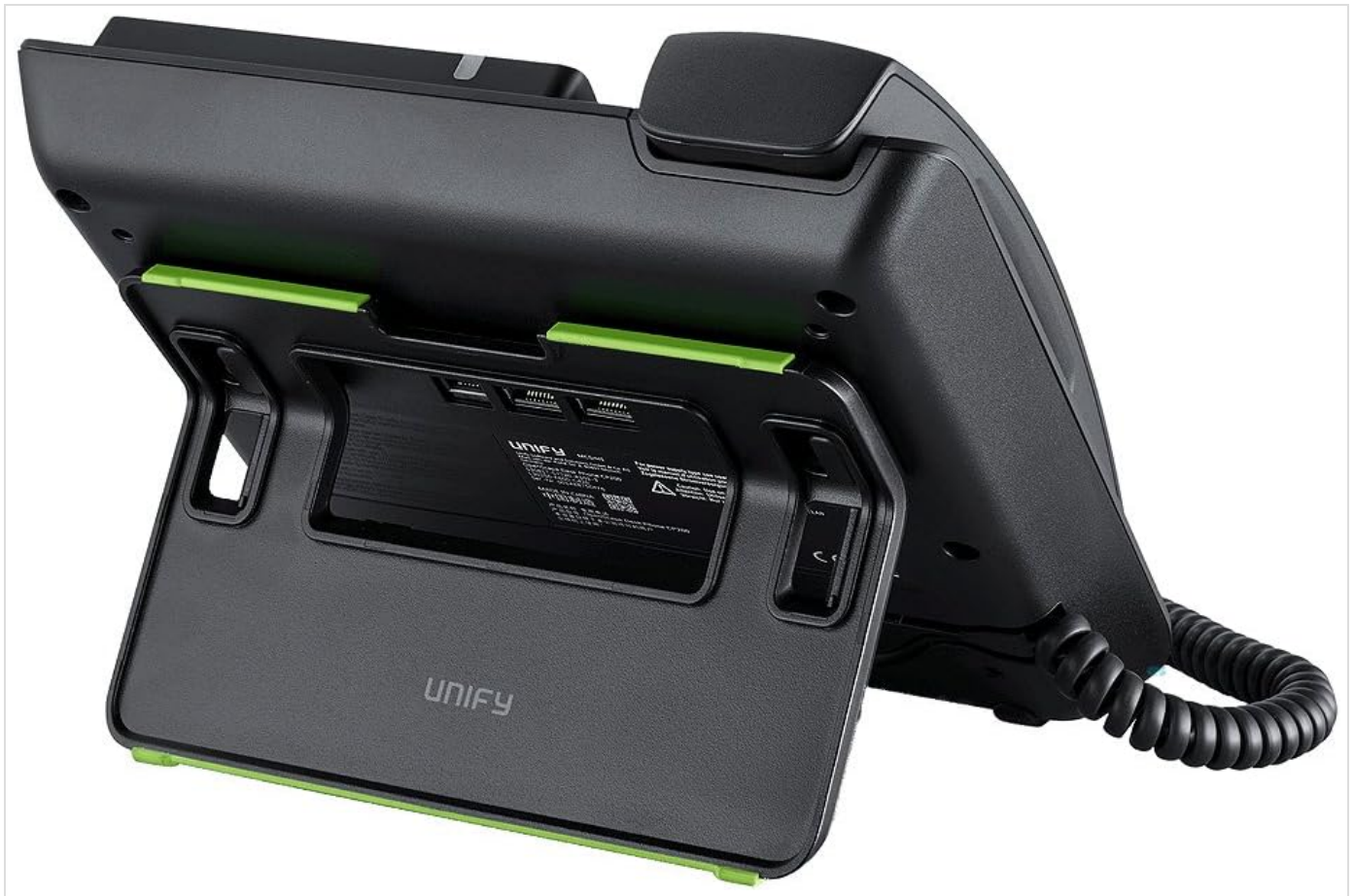
Figure 3.1: Rear view of the phone, illustrating the ports for handset, Ethernet, and power connections. The integrated stand is also visible.
