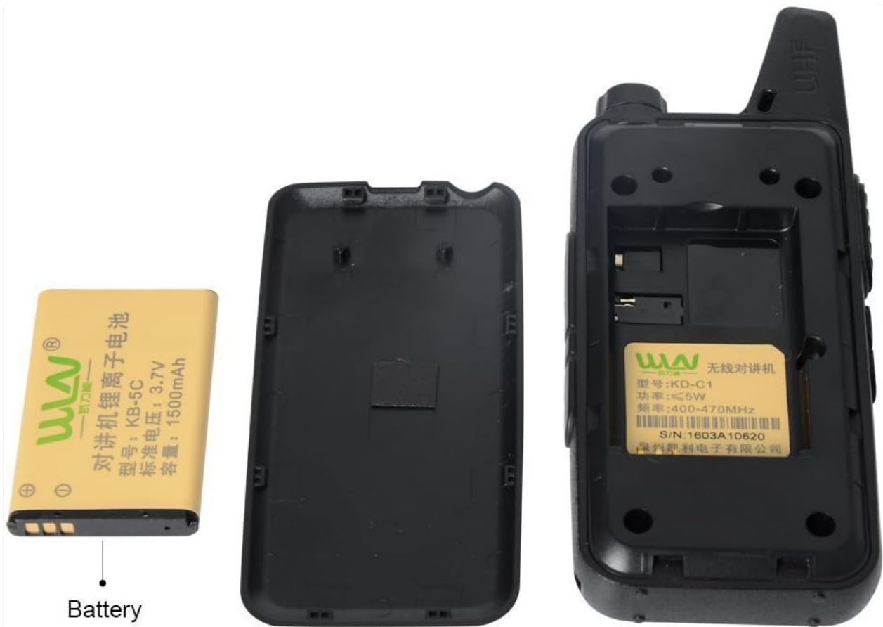
Figure 4: Disassembled view of the KD-C1 showing the battery, battery compartment, and back cover, illustrating battery installation.
