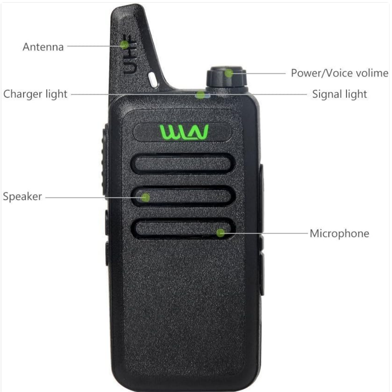
Figure 1: Labeled components of the KD-C1 Walkie Talkie, showing the antenna, power/voice volume knob, signal light, charger light, speaker, and microphone.
