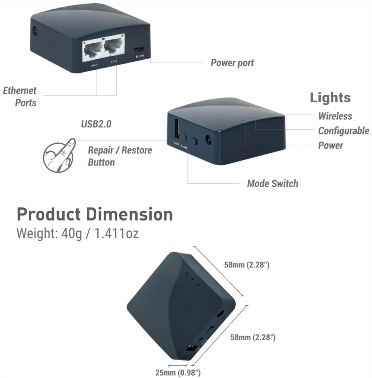
Figure 2: Device Layout and Dimensions. This image illustrates the router's ports (WAN, LAN, Power, USB 2.0), buttons (Repair/Restore, Mode Switch), and indicator lights (Wireless, Configurable, Power). The dimensions are shown as 58mm (2.28") x 58mm (2.28") x 25mm (0.98"), with a weight of 40g (1.41oz).
