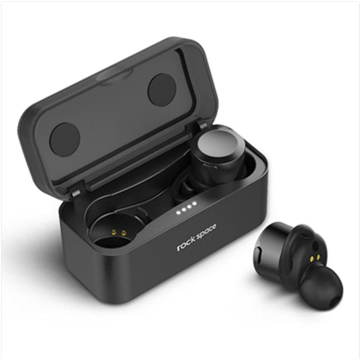
Image 1: The Rock Space EB10 True Wireless Stereo Earphones, with one earbud removed from its charging case, illustrating the compact design and charging contacts.
