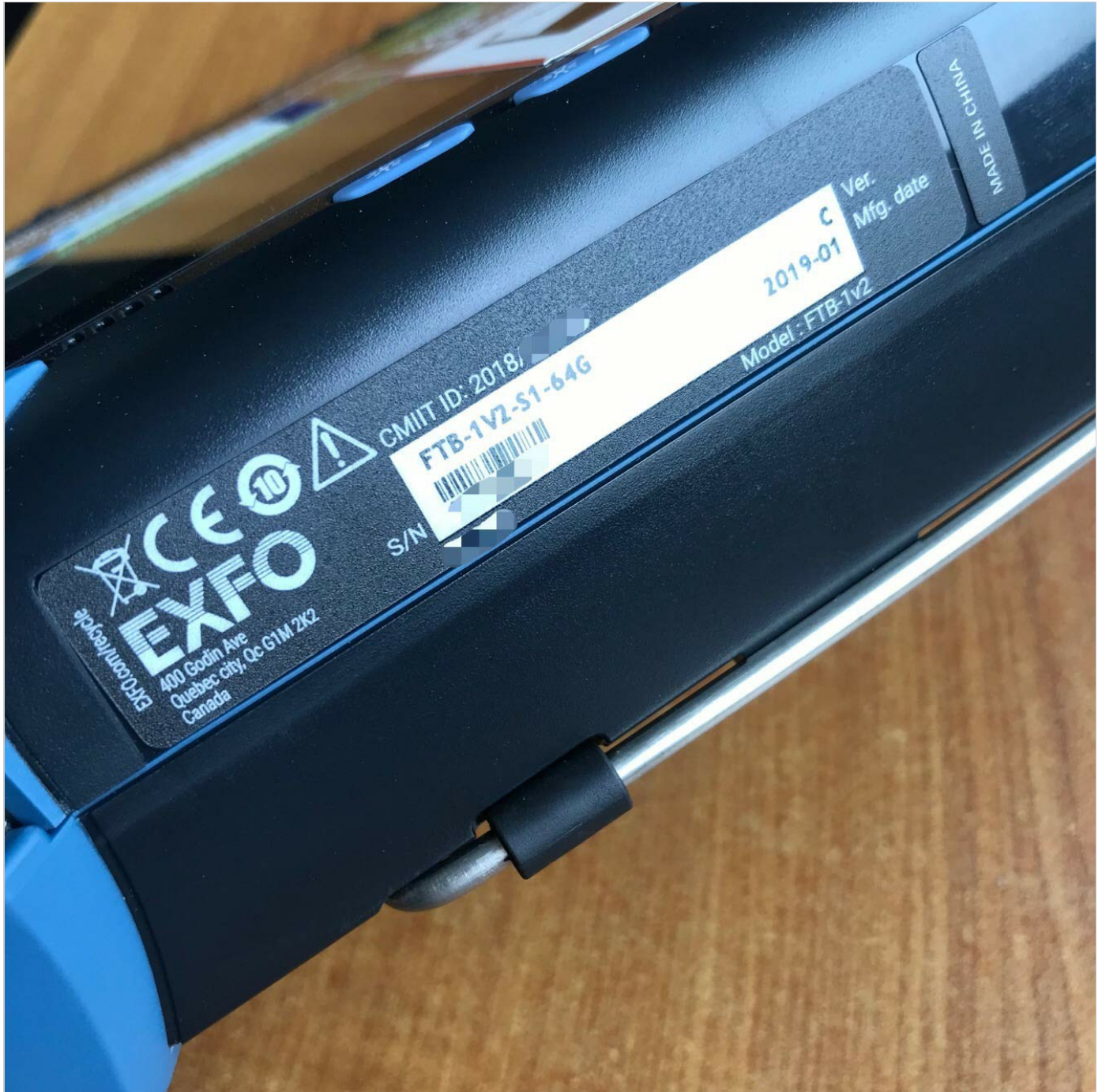
Figure 4.1: Rear view of the EXFO FTB-1V2, displaying important product labels including the serial number, model information (FTB-1V2), manufacturing date, and regulatory compliance marks (CE, CMIT ID), which are crucial for identification and service.
