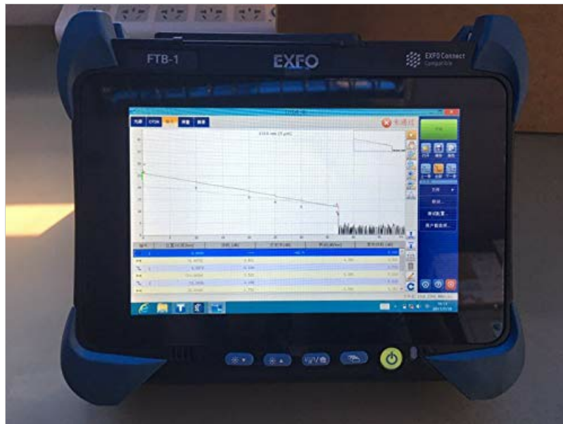
Figure 3.1: The EXFO FTB-1V2 screen showing an Optical Time-Domain Reflectometer (OTDR) trace graph, which is used to characterize optical fibers. The graph displays signal loss over distance, indicating splices, connectors, and fiber breaks.
