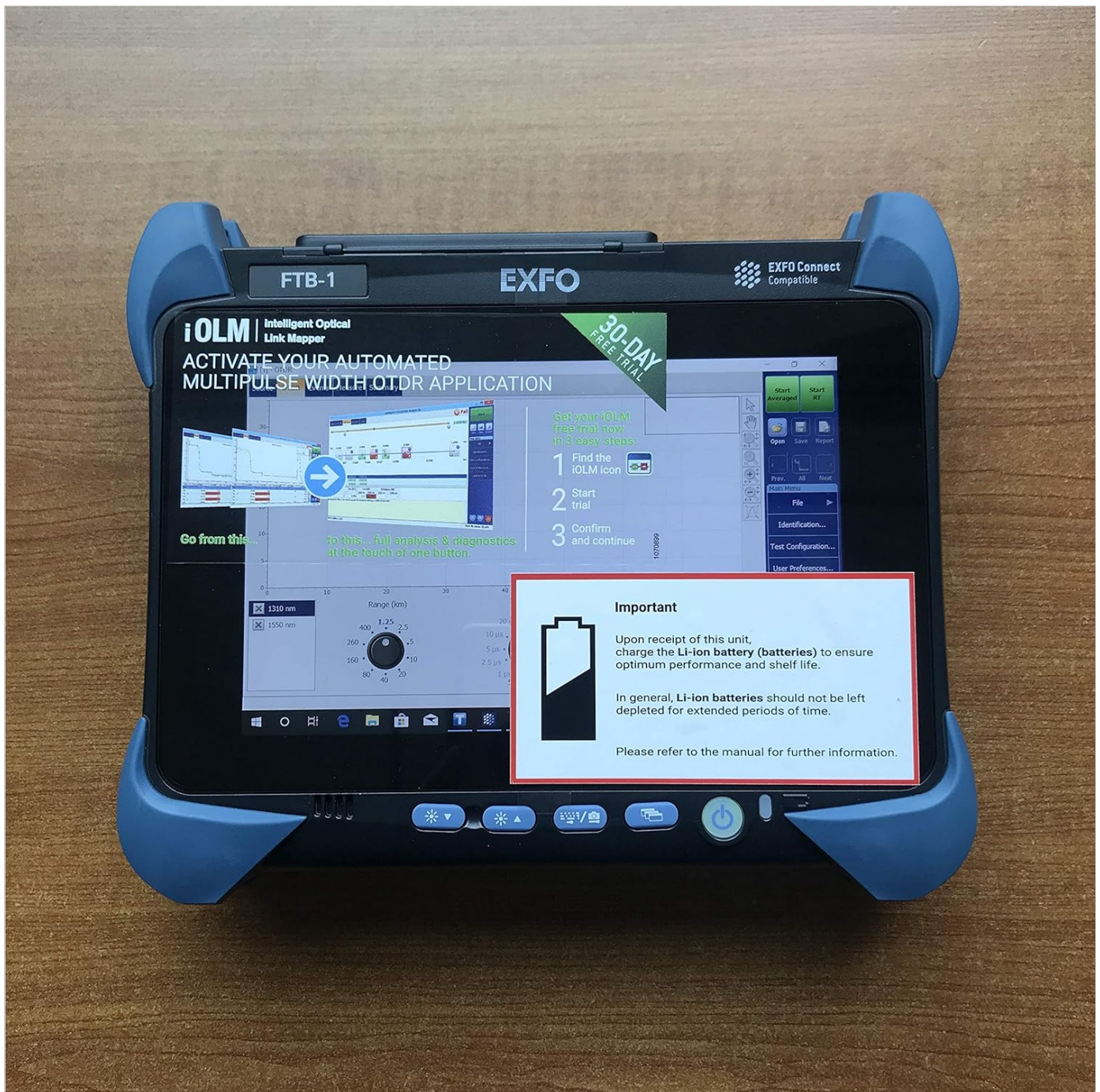
Figure 1.1: Front view of the EXFO FTB-1V2 unit, showing the touchscreen display with an important message regarding battery charging upon receipt to ensure optimal performance and shelf life. It also highlights the iOLM (Intelligent Optical Link Mapper) application.
