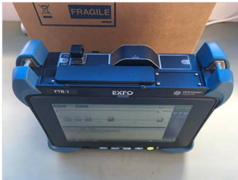
Figure 3.2: Top-down view of the EXFO FTB-1V2, providing a clear perspective of the main display and the top panel where modular components are inserted, emphasizing its adaptable design.
