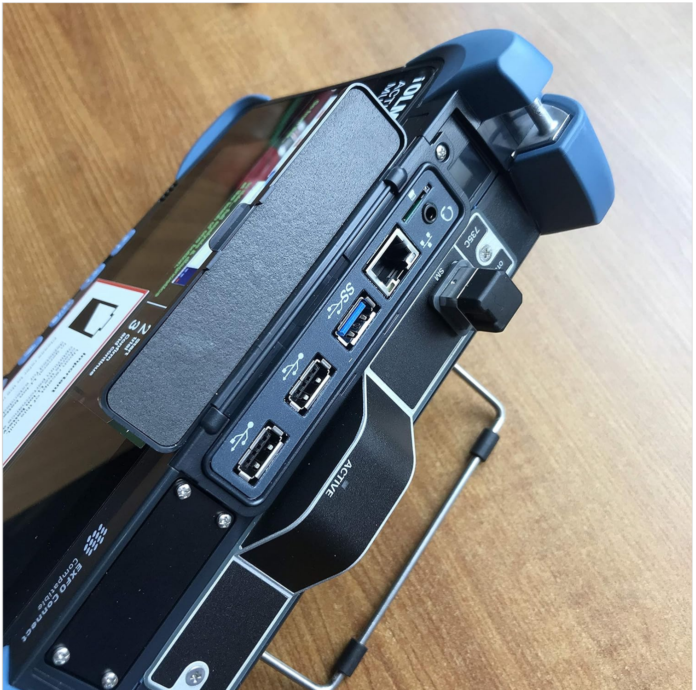
Figure 2.3: Side view of the EXFO FTB-1V2, illustrating the various connectivity ports such as USB (including USB 3.0), Ethernet, and other module-specific interfaces, essential for connecting peripherals and network cables.
