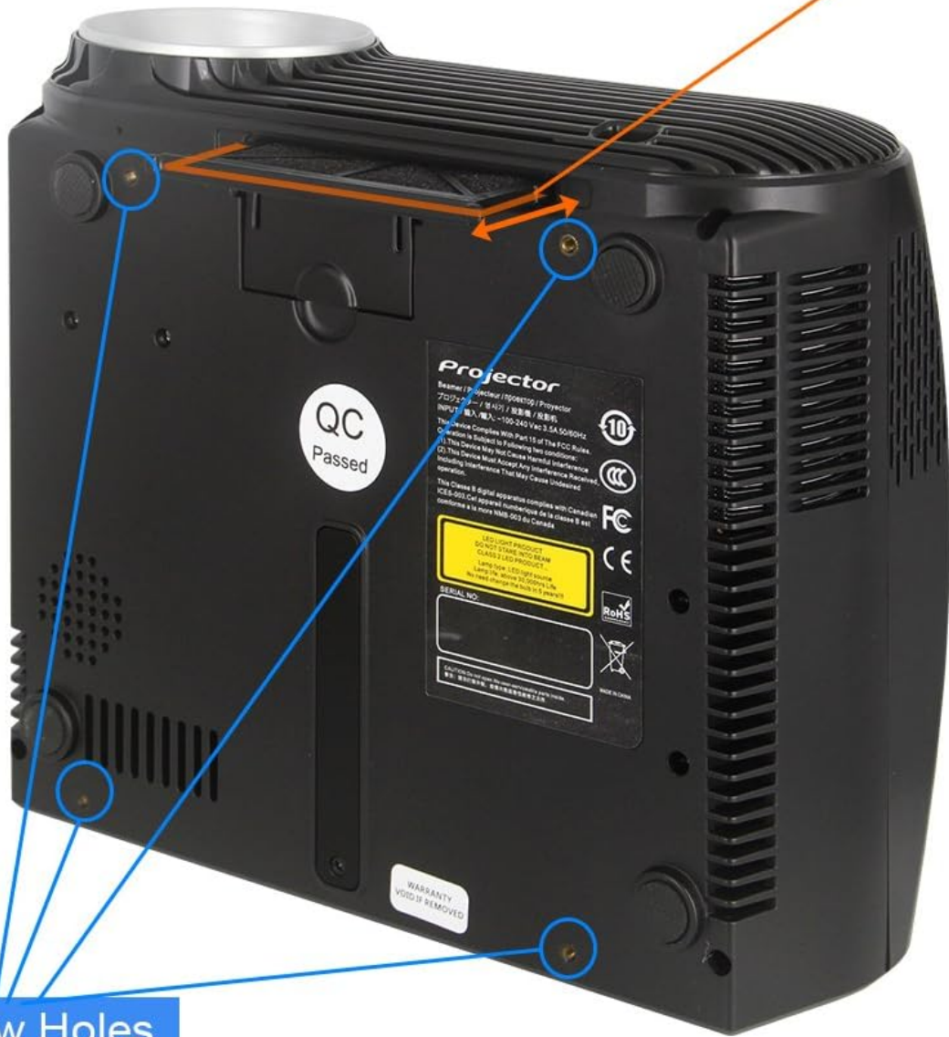
Image 2.3.1: Bottom view of the Newpal NP100 Projector, indicating the locations of the screw holes for mounting.
