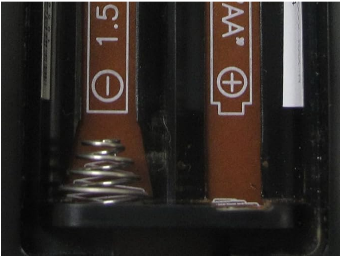
Image: The open battery compartment of the remote control, illustrating where to insert two AA batteries according to their positive and negative terminals.
