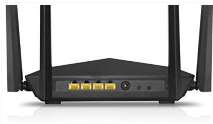
Figure 3.1: Rear view of the router, highlighting the WAN port (often yellow) and multiple LAN ports for wired connections.
