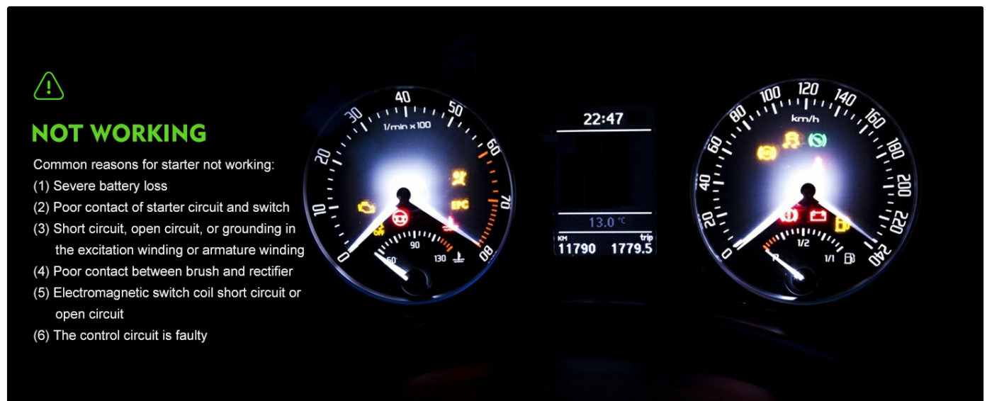
Figure 8.1: Common dashboard indicators and reasons for a starter motor not working.
