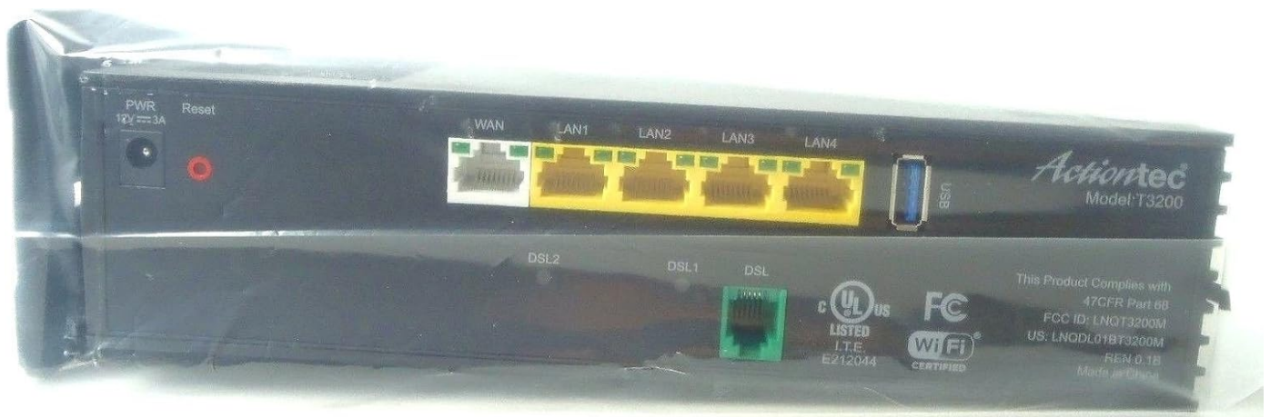
Image: The rear panel of the Actiontec T3200, displaying the power input, reset button, WAN port, four LAN ports, two DSL ports, and a USB port.
