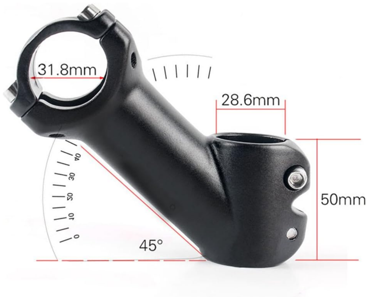
Image 2: The WAKE MTB Stem with key dimensions highlighted, including handlebar diameter (31.8mm), steerer tube diameter (28.6mm), and the 45-degree rise.
