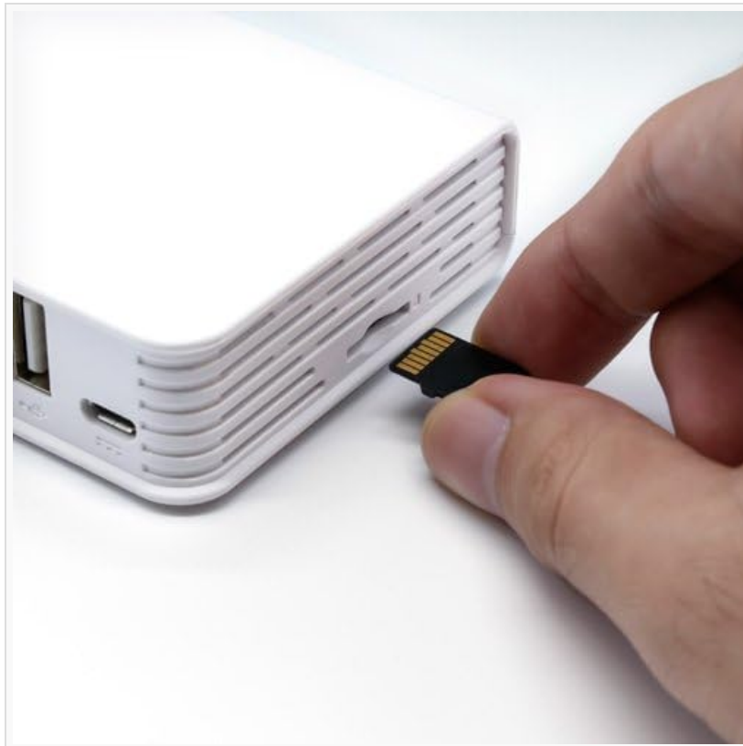
Figure 4.1: Inserting a MicroSD Card
