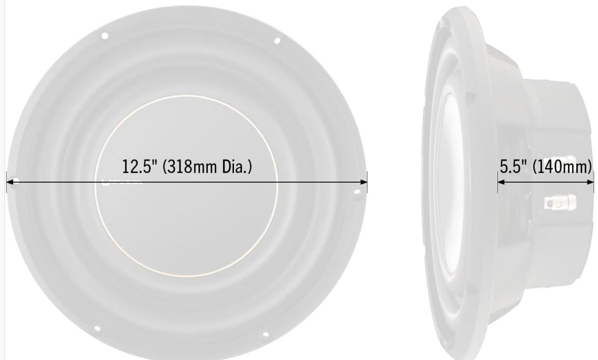
Figure 6: Dimensional diagram of the TS-D12D4 subwoofer, showing its diameter and mounting depth.
